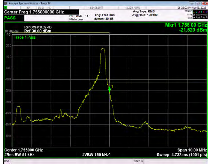
Band4 QPSK BW=5MHz Channel=20375 RB Size=25 Position=#0 Extended
