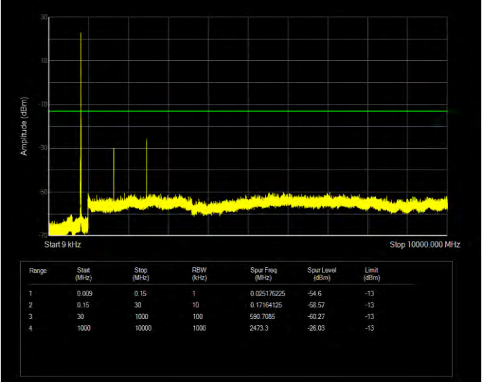
Band5 QPSK BW=3MHz Channel=20415 RB Size=1 Position=#0
