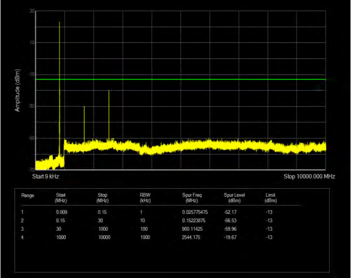
Band5 QPSK BW=10MHz Channel=20525 RB Size=1 Position=#0
