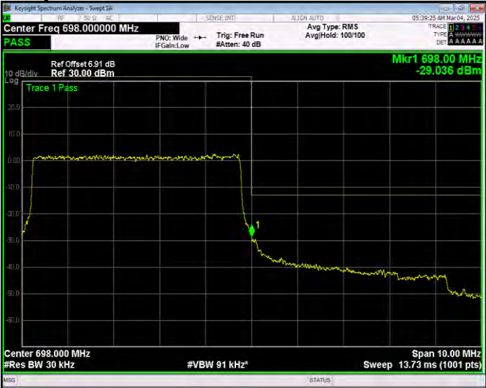
Band71 QPSK BW=5MHz Channel=133447 RB Size=25 Position=#0 Normal
