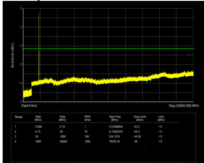
Band2 16QAM BW=10MHz Channel=19150 RB Size=1 Position=#0
