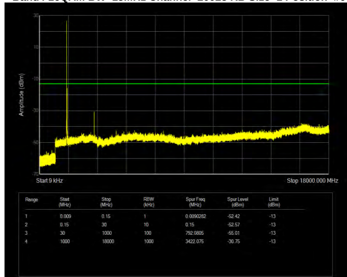
Band4 16QAM BW=15MHz Channel=20025 RB Size=1 Position=#0
