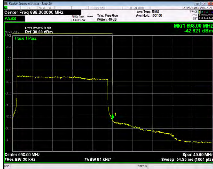
Band71 QPSK BW=5MHz Channel=133147 RB Size=1 Position=#0 Normal
