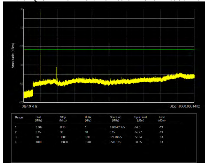
Band4 QPSK BW=5MHz Channel=20375 RB Size=1 Position=#0
