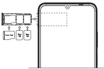
Please insert a Nano SIM card on the Slot 1, a Nano SIM card on the Slot2 and a micro SD card on the TF card Slot.
