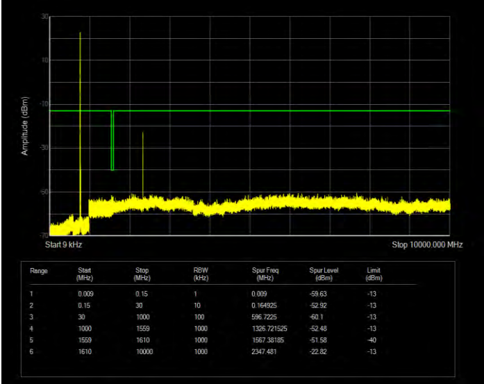
Band17 16QAM BW=10MHz Channel=23780 RB Size=1 Position=#0
