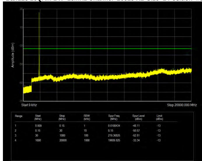
Band25 16QAM BW=20MHz Channel=26140 RB Size=1 Position=#0
