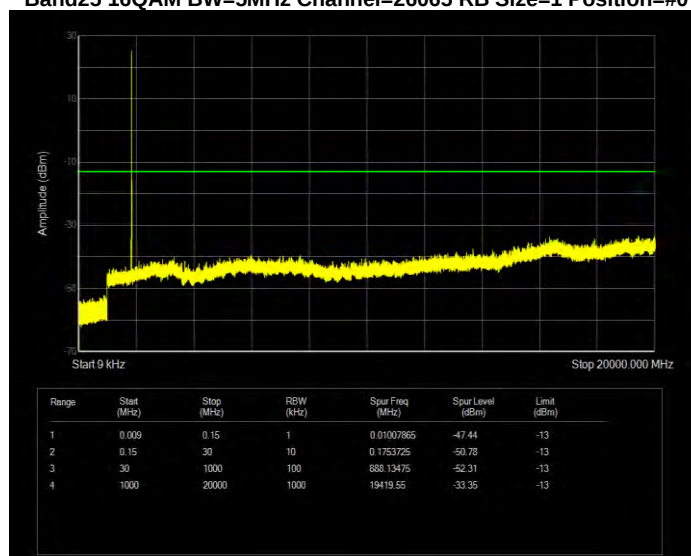
Band25 16QAM BW=5MHz Channel=26365 RB Size=1 Position=#0
