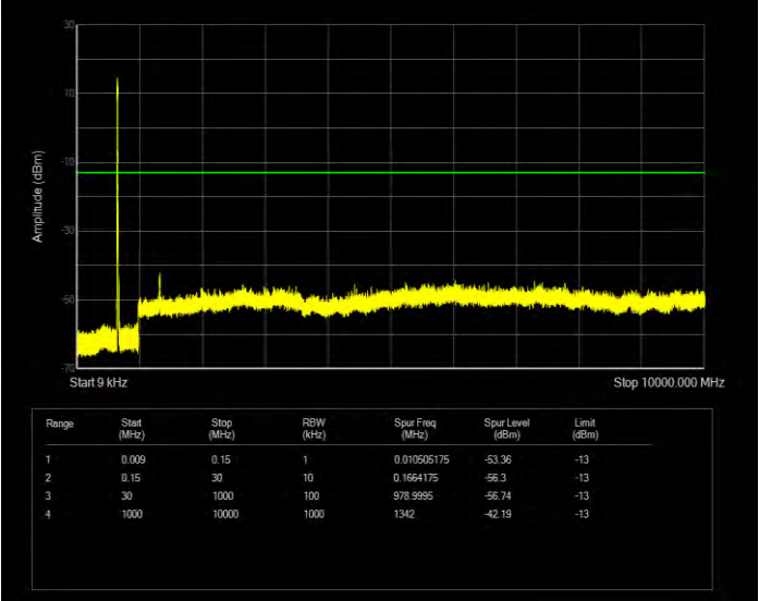
Band71 QPSK BW=10MHz Channel=133297 RB Size=50 Position=#0
