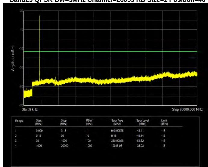
Band25 QPSK BW=3MHz Channel=26365 RB Size=1 Position=#0
