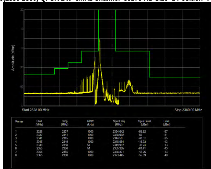
Band40(2350-2360) QPSK BW=5MHz Channel=39175 RB Size=25 Position=#0 Extended
