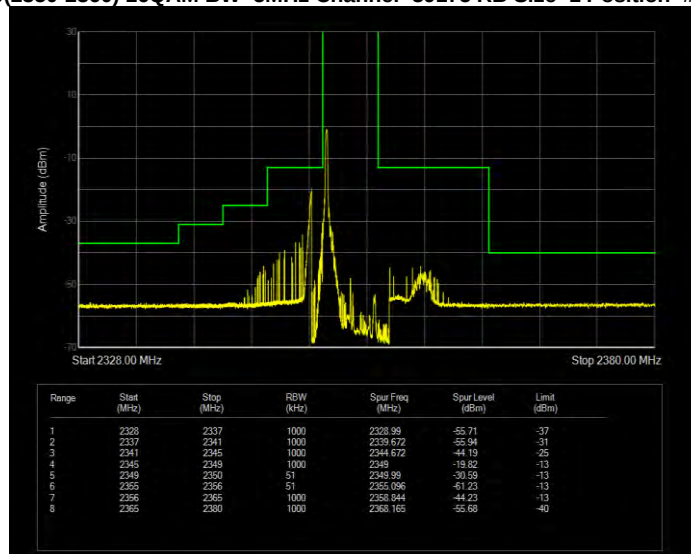
Band40(2350-2360) 16QAM BW=5MHz Channel=39175 RB Size=25 Position=#0 Extended
