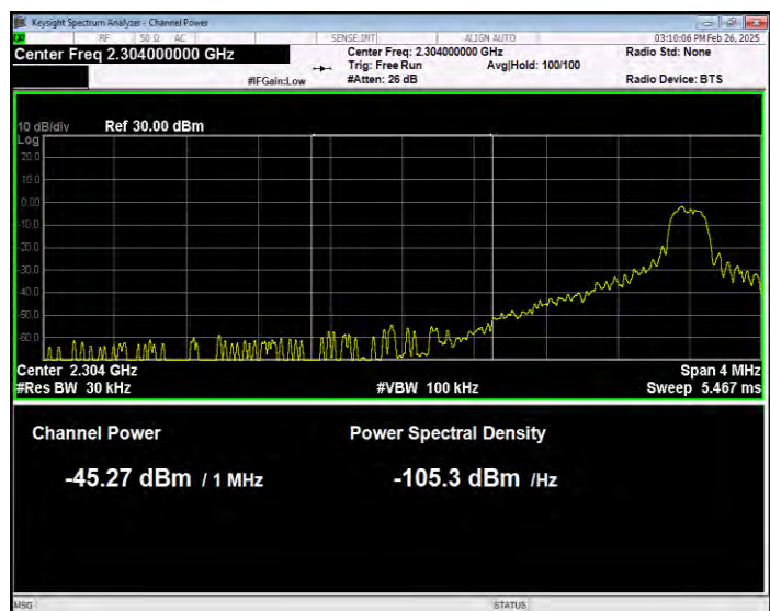
Band40(2305-2315) QPSK BW=10MHz Channel=38750 RB Size=1 Position=#0 Normal
