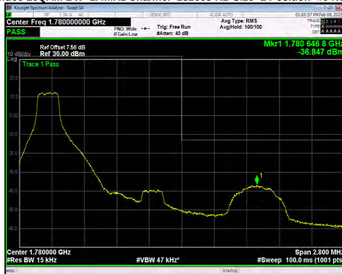
Band66 16QAM BW=1.4MHz Channel=132665 RB Size=1 Position=#Max Extended
