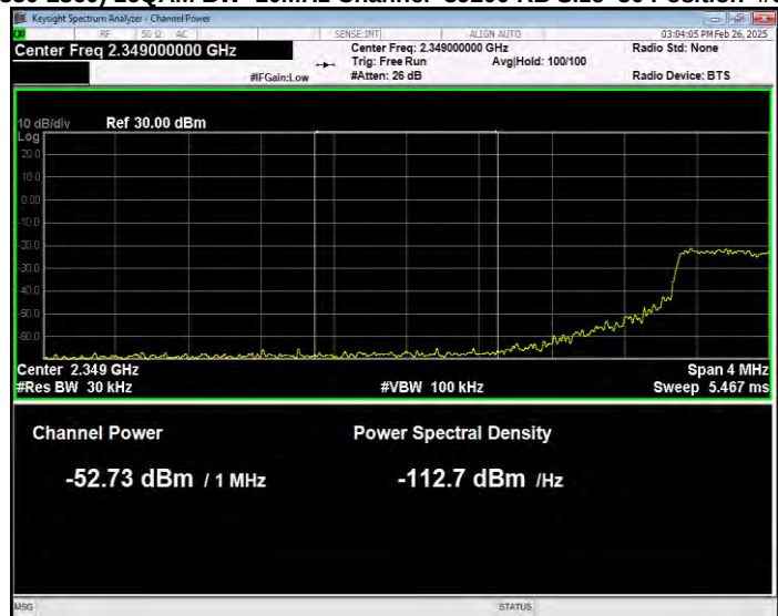
Band40(2350-2360) 16QAM BW=10MHz Channel=39200 RB Size=50 Position=#0 Normal
