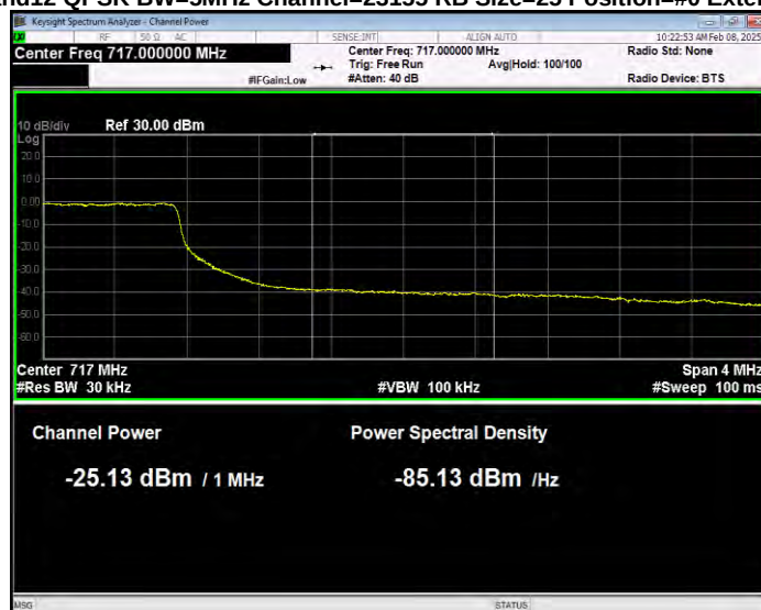
Band12 QPSK BW=5MHz Channel=23155 RB Size=25 Position=#0 Normal
