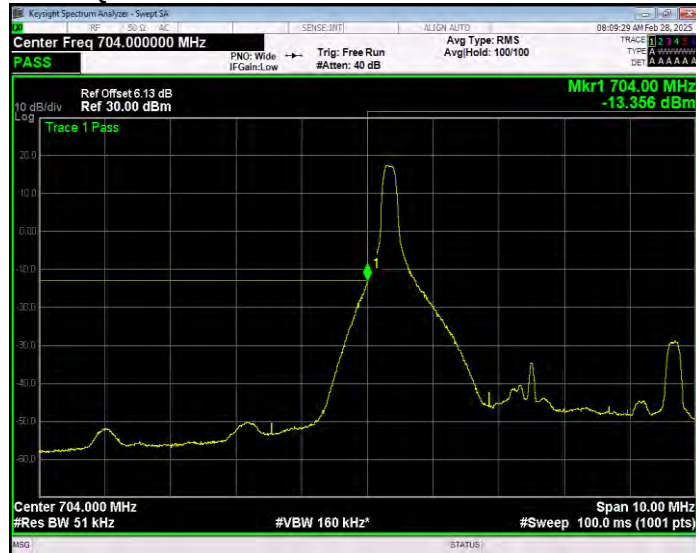
Band17 16QAM BW=5MHz Channel=23755 RB Size=1 Position=#Max Extended
