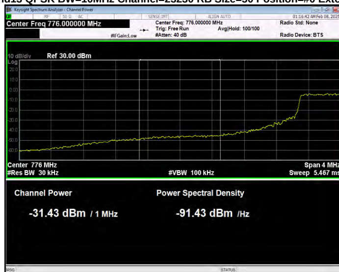
Band13 QPSK BW=10MHz Channel=23230 RB Size=50 Position=#0 Normal
