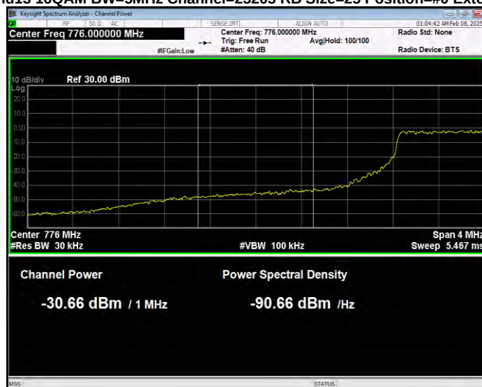
Band13 16QAM BW=5MHz Channel=23205 RB Size=25 Position=#0 Normal
