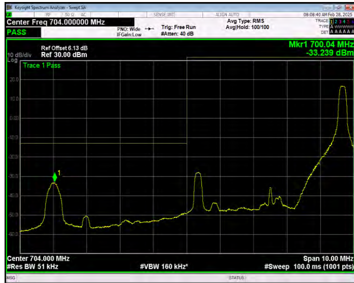
Band17 QPSK BW=5MHz Channel=23755 RB Size=25 Position=#0 Extended
