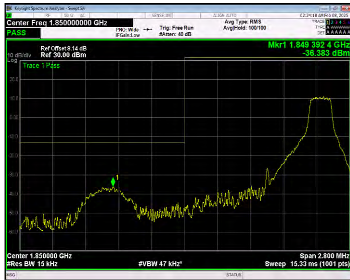
Band25 16QAM BW=1.4MHz Channel=26047 RB Size=6 Position=#0 Extended
