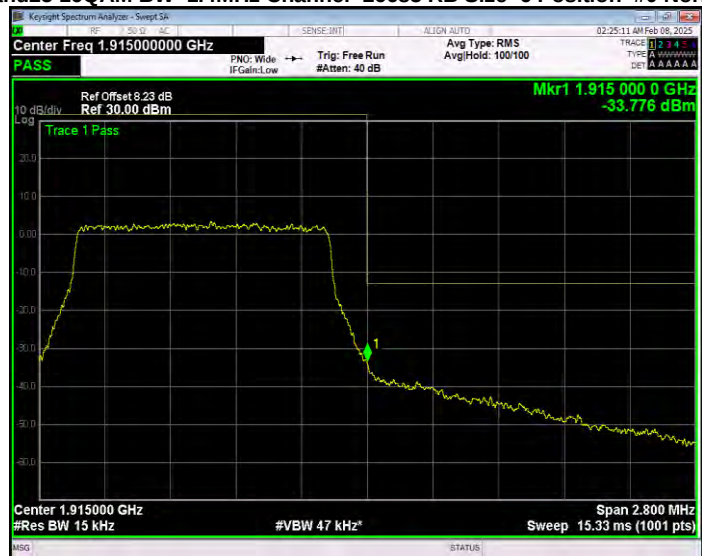
Band25 16QAM BW=10MHz Channel=26090 RB Size=1 Position=#0 Extended
