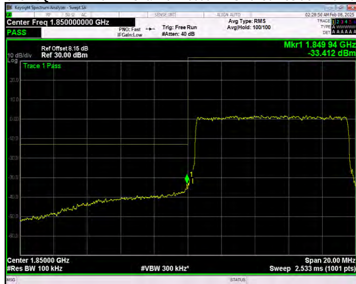
Band25 16QAM BW=10MHz Channel=26640 RB Size=1 Position=#0 Extended
