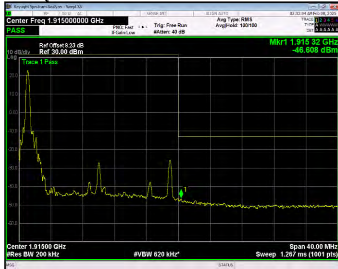
Band25 16QAM BW=20MHz Channel=26590 RB Size=1 Position=#Max Extended
