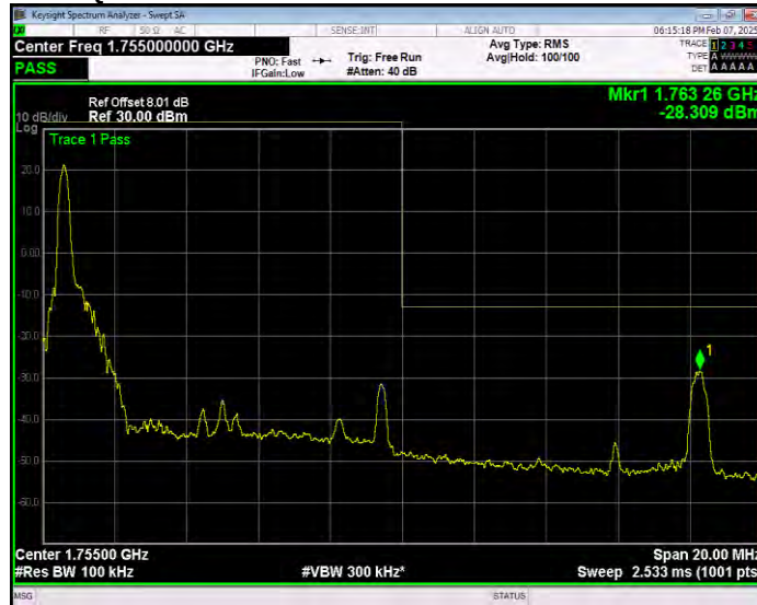
Band4 16QAM BW=10MHz Channel=20350 RB Size=1 Position=#Max Extended
