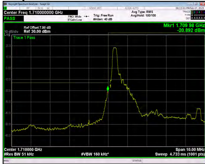
Band4 QPSK BW=5MHz Channel=19975 RB Size=1 Position=#Max Extended
