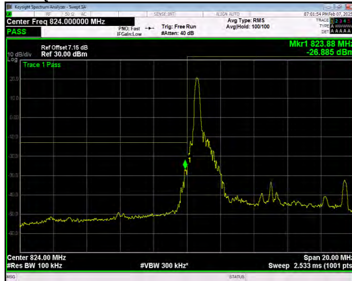
Band5 16QAM BW=10MHz Channel=20450 RB Size=1 Position=#Max Extended
