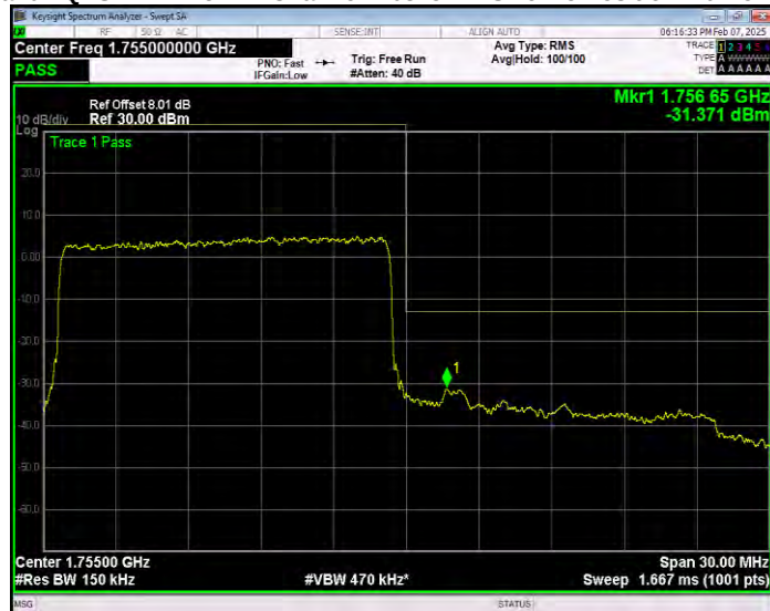
Band4 QPSK BW=20MHz Channel=20050 RB Size=1 Position=#0 Extended
