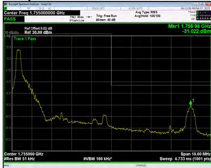
Band4 16QAM BW=5MHz Channel=20375 RB Size=1 Position=#Max Extended
