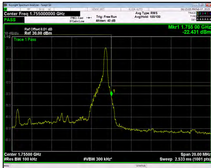
Band4 QPSK BW=10MHz Channel=20350 RB Size=50 Position=#0 Extended
