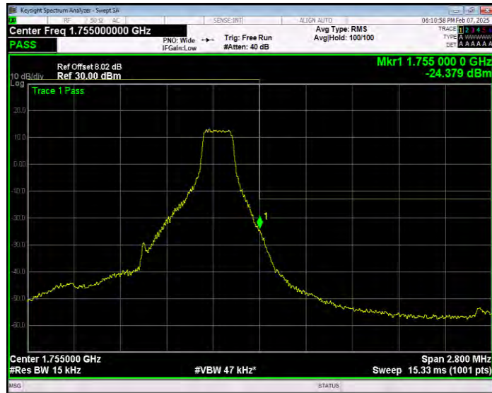
Band4 QPSK BW=1.4MHz Channel=20393 RB Size=6 Position=#0 Extended
