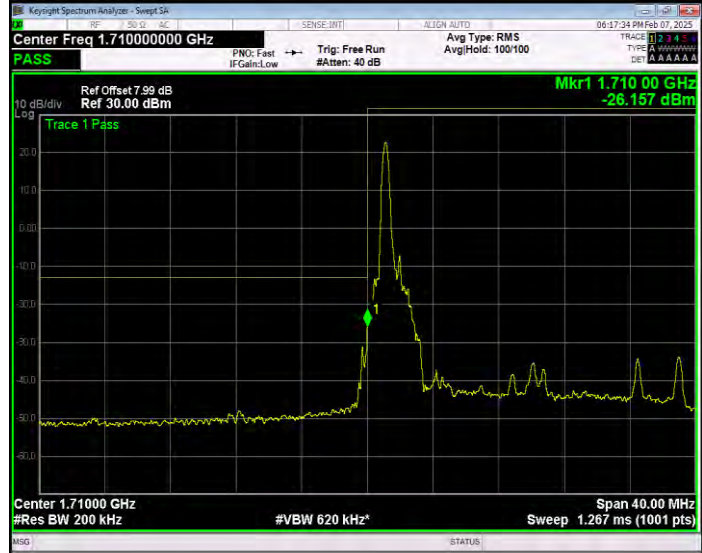
Band4 QPSK BW=20MHz Channel=20050 RB Size=1 Position=#Max Extended
