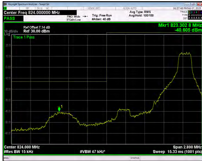
Band5 16QAM BW=1.4MHz Channel=20407 RB Size=6 Position=#0 Extended
