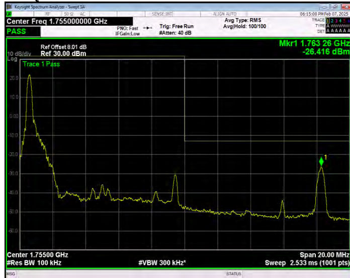
Band4 QPSK BW=10MHz Channel=20350 RB Size=1 Position=#Max Extended
