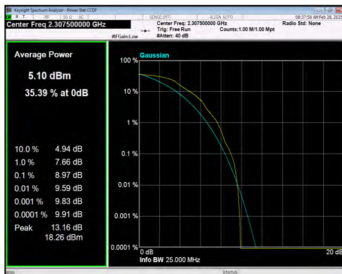
Band40(2305-2315) QPSK BW=5MHz Channel=38750 RB Size=1 Position=#0
