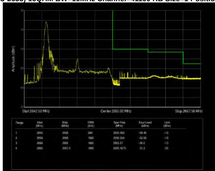
Band41(2535-2655) 16QAM BW=10MHz Channel=41190 RB Size=1 Position=#Max Extended
