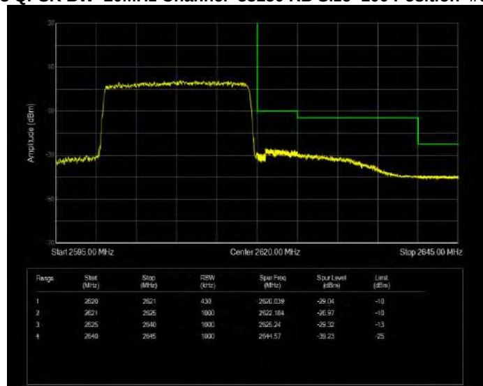
Band38 QPSK BW=5MHz Channel=37775 RB Size=1 Position=#0 Extended
