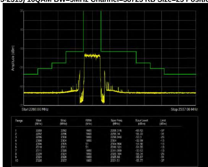
Band40(2305-2315) 16QAM BW=5MHz Channel=38775 RB Size=1 Position=#0 Extended
