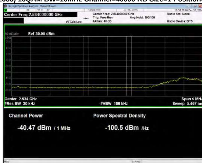
Band41(2535-2655) 16QAM BW=10MHz Channel=40090 RB Size=1 Position=#Max Normal
