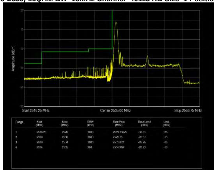
Band41(2535-2655) 16QAM BW=15MHz Channel=40115 RB Size=1 Position=#Max Extended
