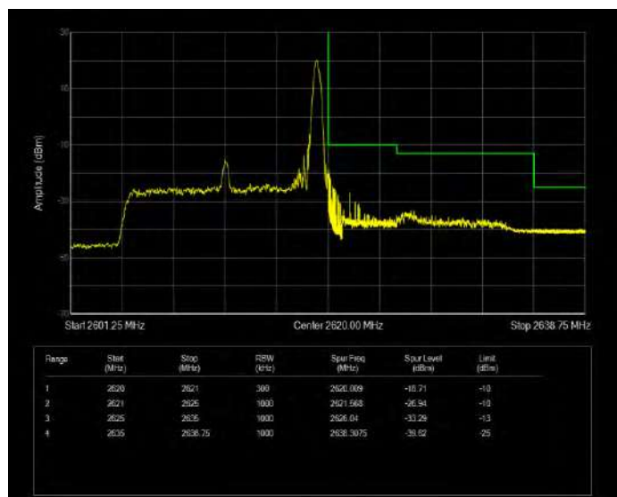
Band38 QPSK BW=15MHz Channel=38175 RB Size=75 Position=#0 Extended
