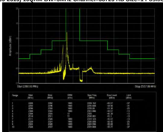
Band40(2305-2315) 16QAM BW=5MHz Channel=38725 RB Size=25 Position=#0 Extended
