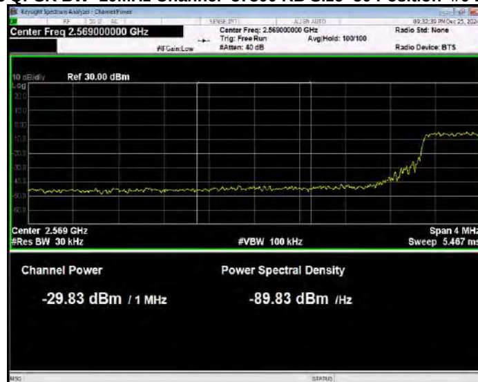
Band38 QPSK BW=10MHz Channel=37800 RB Size=50 Position=#0 Normal
