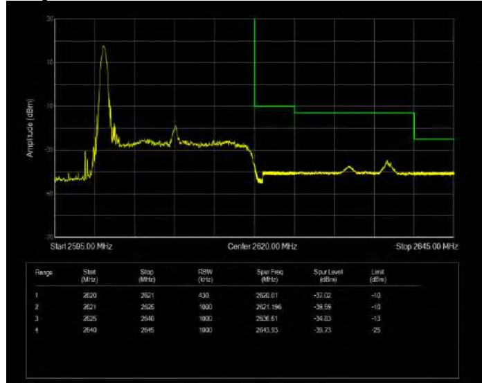
Band38 16QAM BW=20MHz Channel=38150 RB Size=1 Position=#Max Extended
