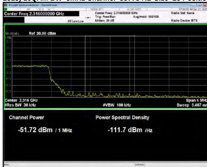
Band40(2305-2315) 16QAM BW=5MHz Channel=38775 RB Size=25 Position=#0 Normal
