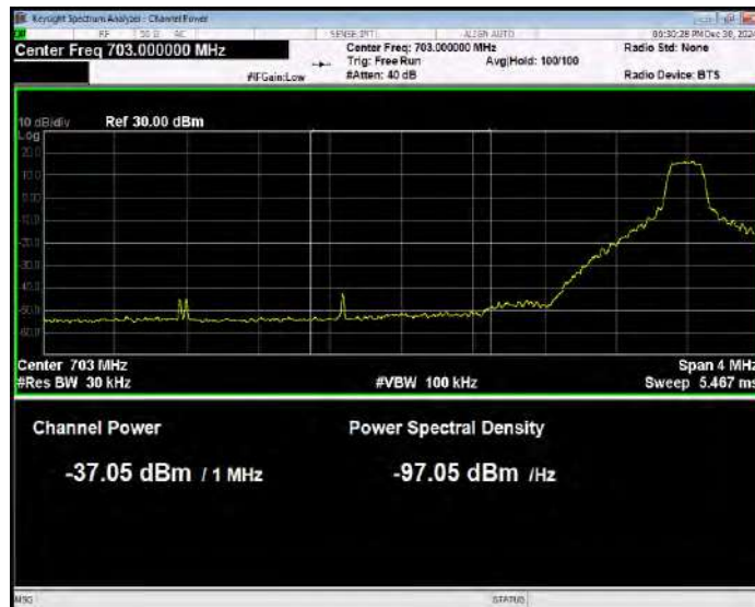
Band17 QPSK BW=10MHz Channel=23780 RB Size=1 Position=#0 Normal
