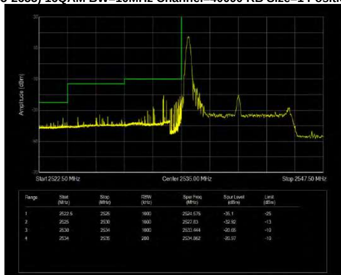
Band41(2535-2655) 16QAM BW=10MHz Channel=40090 RB Size=1 Position=#Max Extended
