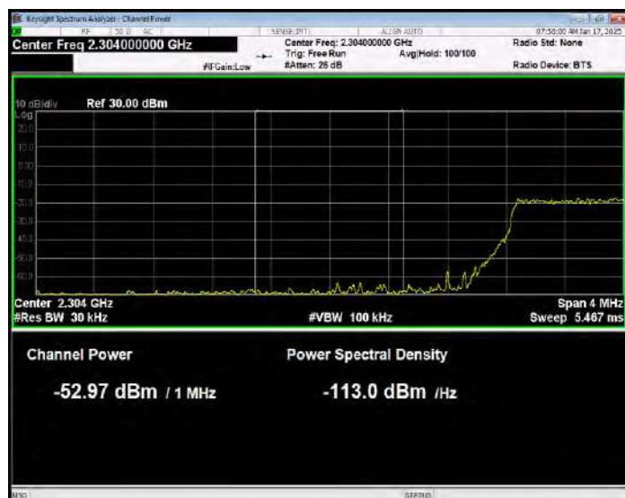
Band40(2305-2315) 16QAM BW=5MHz Channel=38725 RB Size=25 Position=#0 Normal
