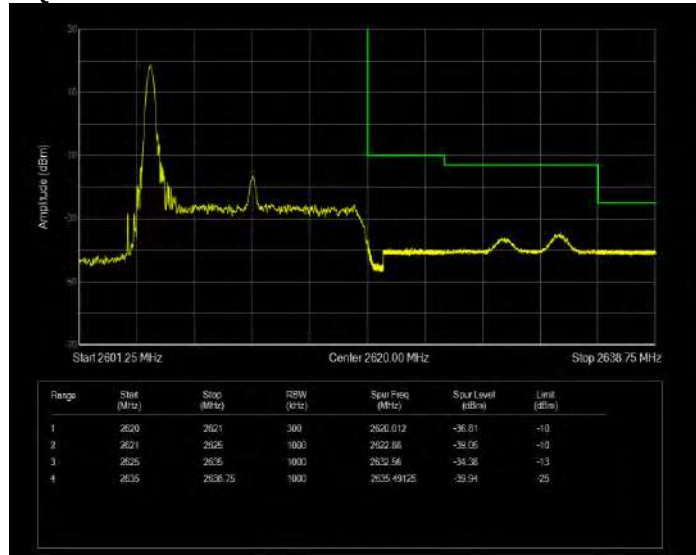
Band38 QPSK BW=15MHz Channel=38175 RB Size=1 Position=#Max Extended
