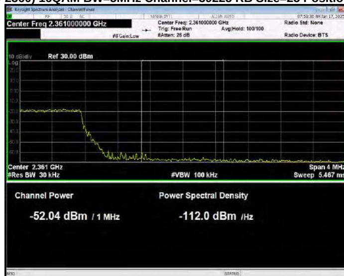
Band40(2350-2360) 16QAM BW=5MHz Channel=39225 RB Size=25 Position=#0 Normal
