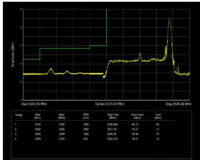
Band38 QPSK BW=20MHz Channel=37850 RB Size=100 Position=#0 Extended
