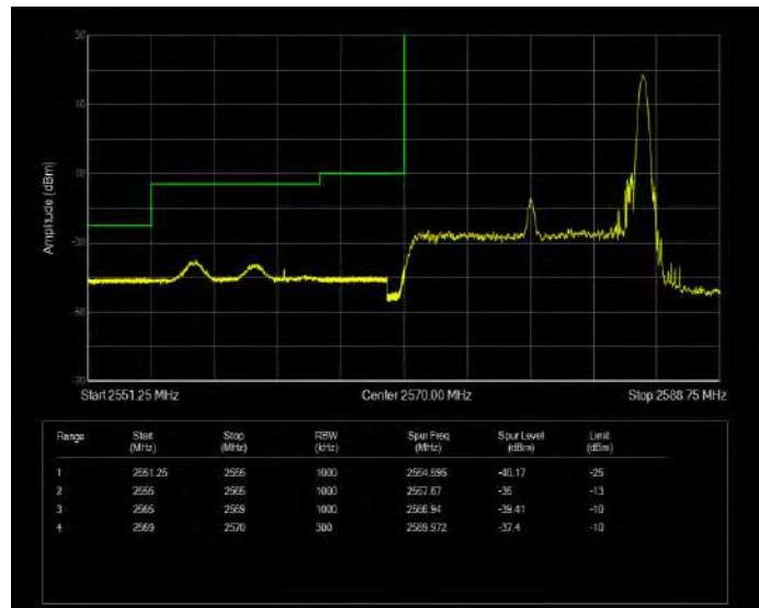
Band38 16QAM BW=15MHz Channel=37825 RB Size=75 Position=#0 Extended
