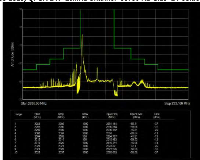
Band40(2305-2315) QPSK BW=10MHz Channel=38750 RB Size=50 Position=#0 Extended
