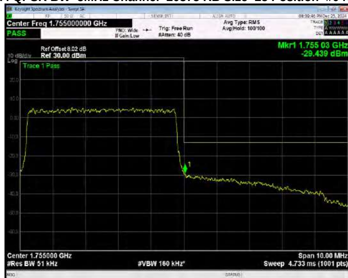
Band5 16QAM BW=1.4MHz Channel=20407 RB Size=1 Position=#0 Extended
