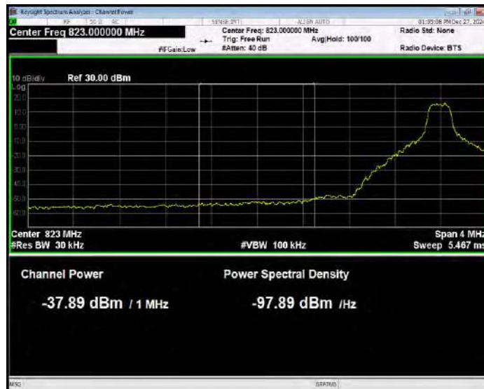
Band5 QPSK BW=10MHz Channel=20450 RB Size=1 Position=#0 Normal
