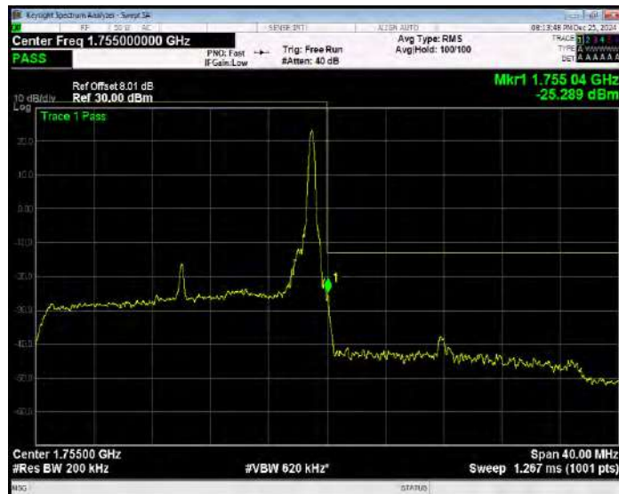
Band4 QPSK BW=20MHz Channel=20300 RB Size=100 Position=#0 Extended
