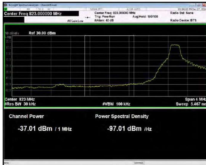
Band5 16QAM BW=5MHz Channel=20425 RB Size=1 Position=#0 Normal
