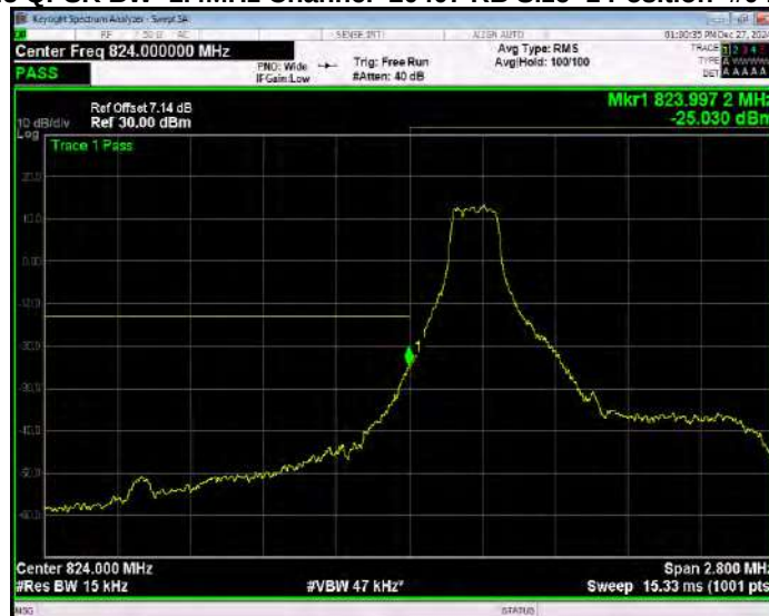
Band5 QPSK BW=1.4MHz Channel=20407 RB Size=1 Position=#Max Extended
