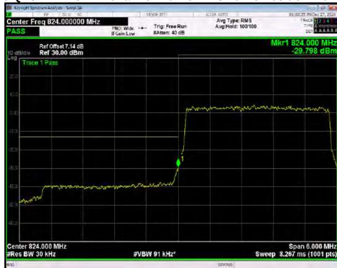
Band5 QPSK BW=3MHz Channel=20635 RB Size=1 Position=#0 Extended
