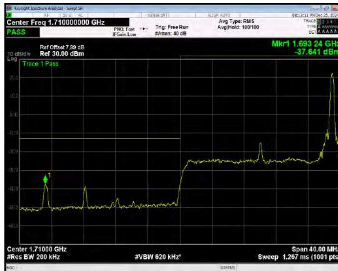
Band4 QPSK BW=20MHz Channel=20050 RB Size=100 Position=#0 Extended
