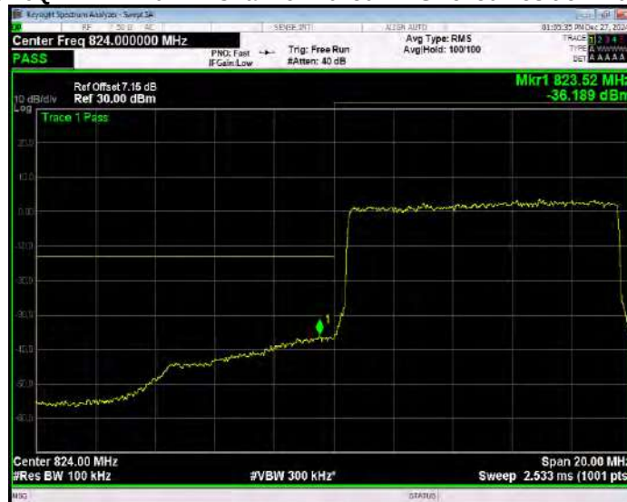
Band5 16QAM BW=10MHz Channel=20600 RB Size=1 Position=#0 Extended
