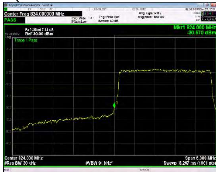
Band5 16QAM BW=3MHz Channel=20635 RB Size=1 Position=#0 Extended
