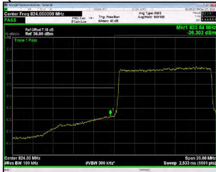
Band5 QPSK BW=10MHz Channel=20600 RB Size=1 Position=#0 Extended
