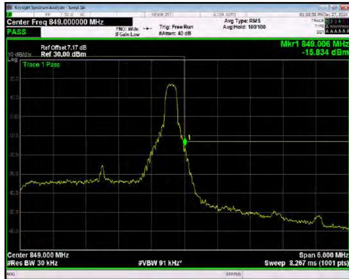
Band5 QPSK BW=3MHz Channel=20635 RB Size=15 Position=#0 Extended
