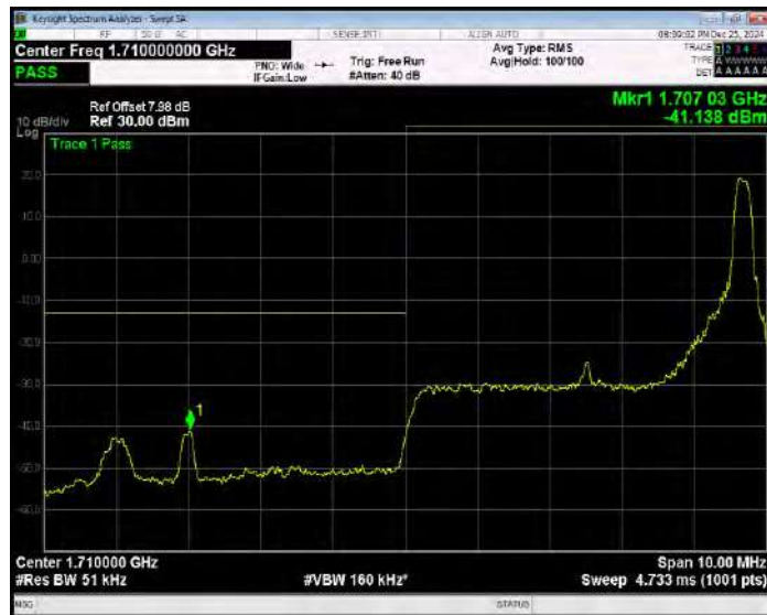
Band4 QPSK BW=5MHz Channel=19975 RB Size=25 Position=#0 Extended
