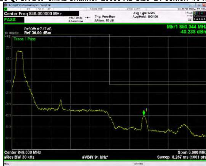
Band5 QPSK BW=3MHz Channel=20635 RB Size=1 Position=#Max Extended
