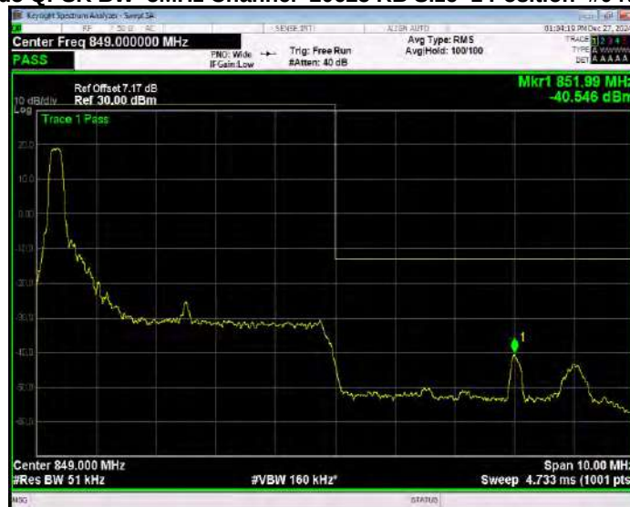
Band5 QPSK BW=5MHz Channel=20625 RB Size=1 Position=#Max Extended
