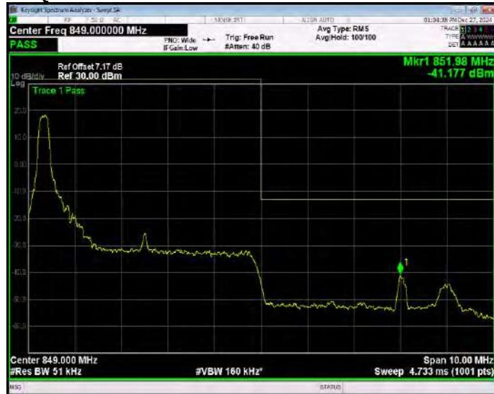
Band5 16QAM BW=5MHz Channel=20625 RB Size=1 Position=#Max Extended
