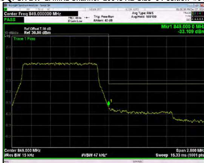
Band5 QPSK BW=10MHz Channel=20450 RB Size=1 Position=#0 Extended
