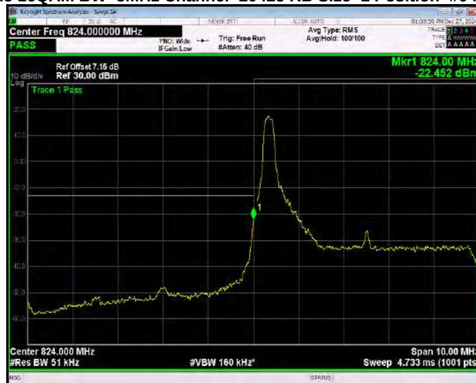
Band5 16QAM BW=5MHz Channel=20425 RB Size=1 Position=#Max Extended
