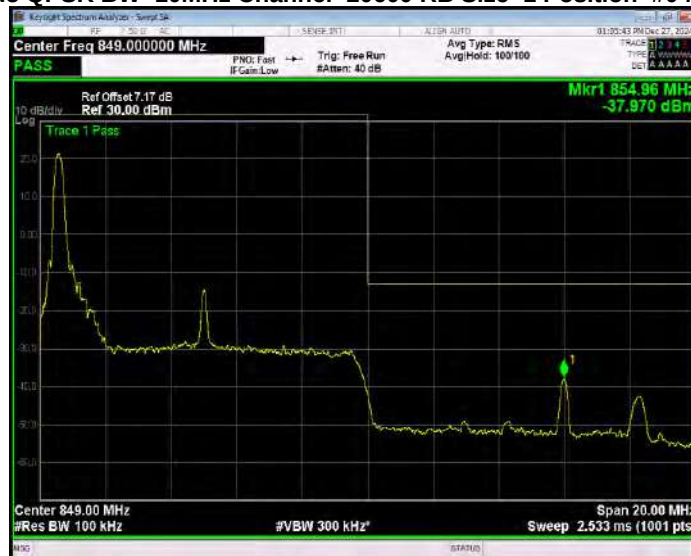
Band5 QPSK BW=10MHz Channel=20600 RB Size=1 Position=#Max Extended
