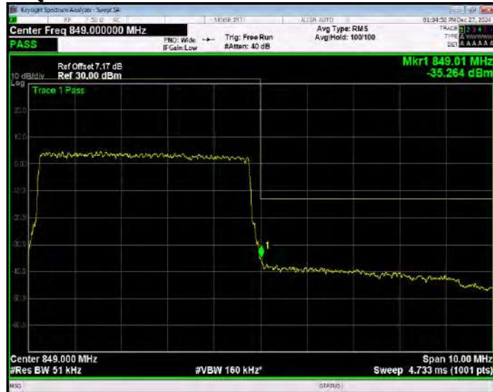
Band5 QPSK BW=1.4MHz Channel=20407 RB Size=1 Position=#0 Extended
