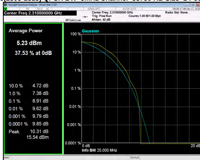
Band40(2305-2315) QPSK BW=5MHz Channel=38775 RB Size=1 Position=#0
