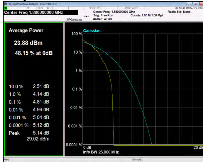
Band2 QPSK BW=20MHz Channel=19100 RB Size=1 Position=#0
