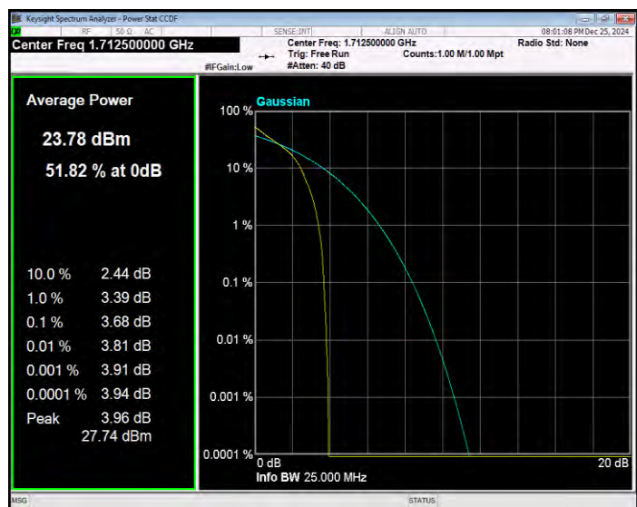
Band4 QPSK BW=5MHz Channel=20175 RB Size=1 Position=#0
