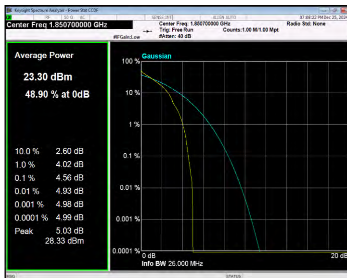
Band2 QPSK BW=1.4MHz Channel=18900 RB Size=1 Position=#0
