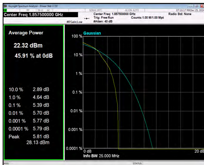
Band2 16QAM BW=15MHz Channel=18900 RB Size=1 Position=#0
