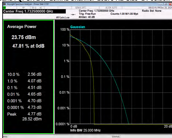
Band4 QPSK BW=20MHz Channel=20300 RB Size=1 Position=#0
