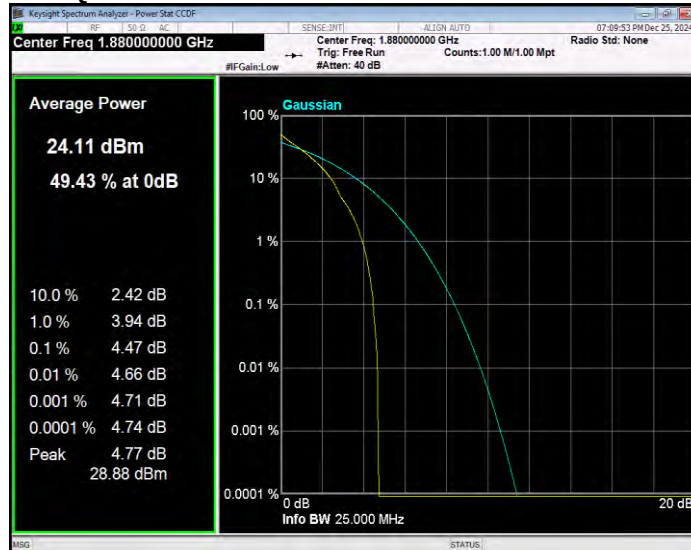
Band2 QPSK BW=10MHz Channel=19150 RB Size=1 Position=#0
