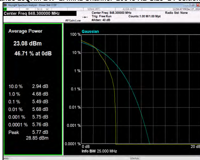
Band5 16QAM BW=10MHz Channel=20450 RB Size=1 Position=#0
