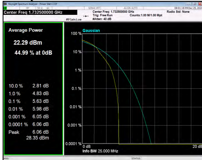
Band4 16QAM BW=5MHz Channel=20375 RB Size=1 Position=#0
