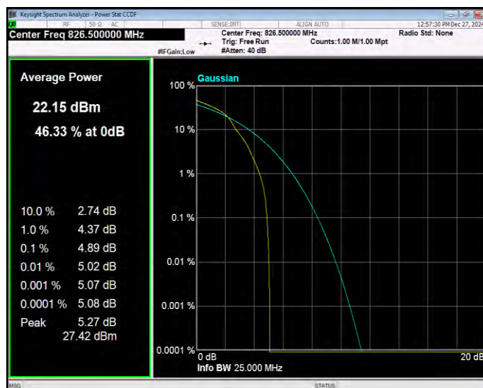
Band5 16QAM BW=5MHz Channel=20525 RB Size=1 Position=#0
