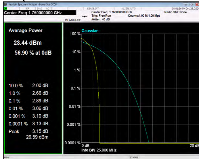
Band4 QPSK BW=15MHz Channel=20025 RB Size=1 Position=#0
