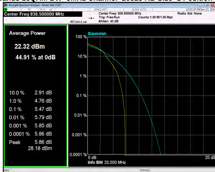
Band5 16QAM BW=5MHz Channel=20625 RB Size=1 Position=#0
