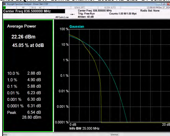
Band5 16QAM BW=10MHz Channel=20600 RB Size=1 Position=#0
