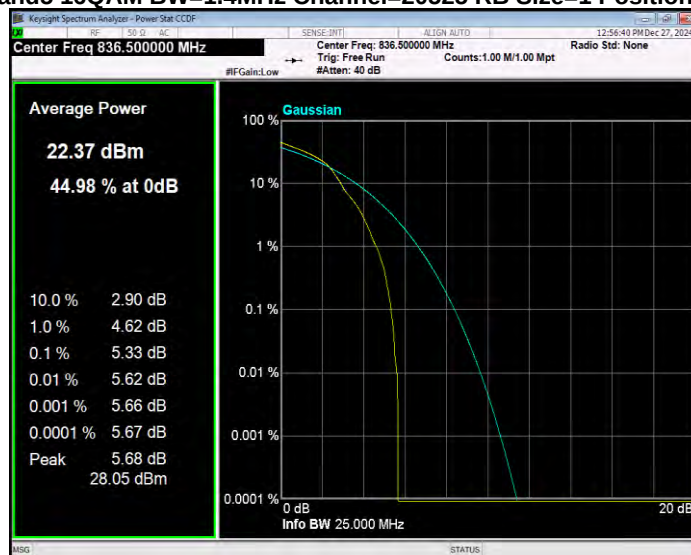
Band5 16QAM BW=1.4MHz Channel=20643 RB Size=1 Position=#0
