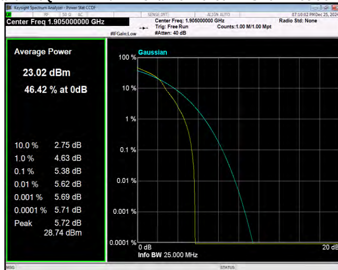
Band2 16QAM BW=15MHz Channel=18675 RB Size=1 Position=#0
