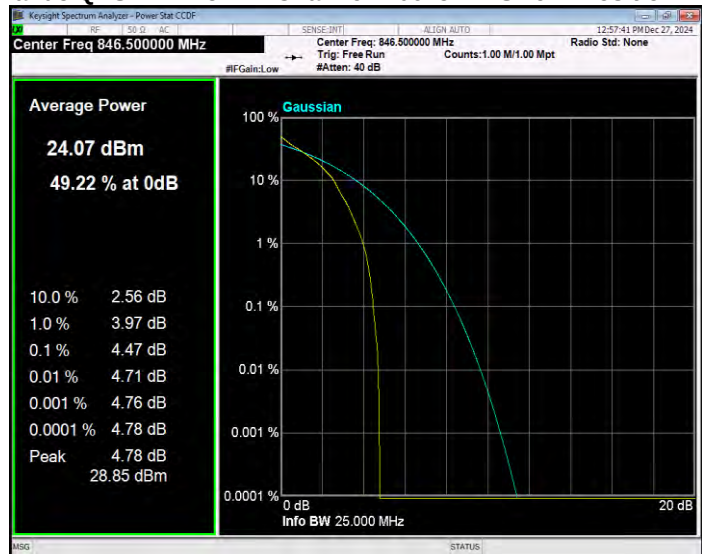
Band7 16QAM BW=10MHz Channel=20800 RB Size=1 Position=#0
