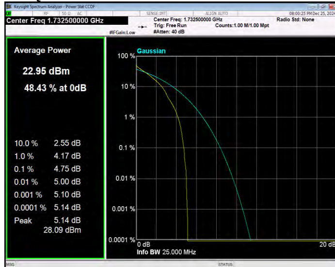
Band4 QPSK BW=1.4MHz Channel=20393 RB Size=1 Position=#0
