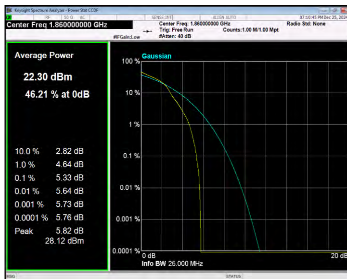
Band2 16QAM BW=20MHz Channel=18900 RB Size=1 Position=#0
