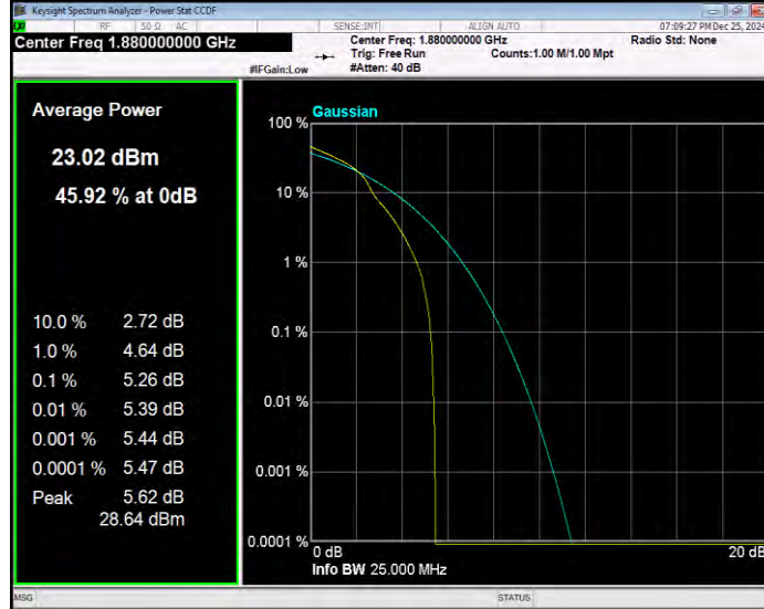
Band2 16QAM BW=5MHz Channel=19175 RB Size=1 Position=#0
