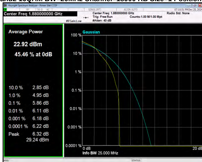
Band2 16QAM BW=20MHz Channel=19100 RB Size=1 Position=#0
