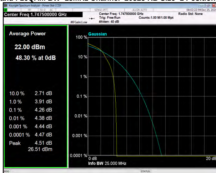
Band4 16QAM BW=20MHz Channel=20050 RB Size=1 Position=#0
