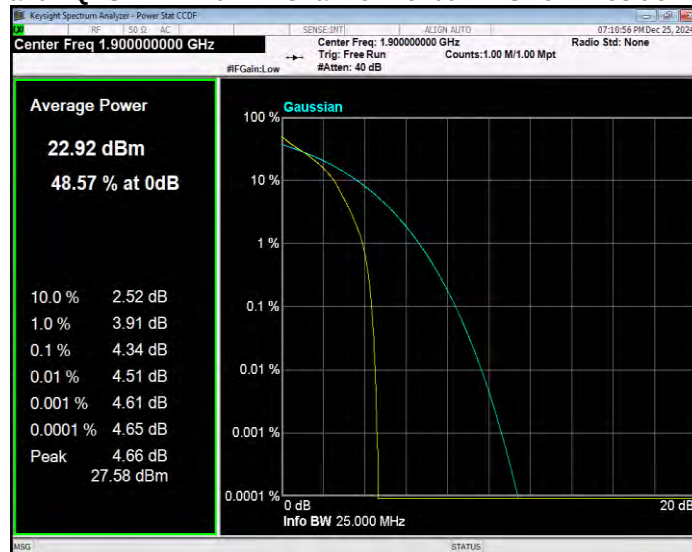
Band2 QPSK BW=3MHz Channel=18615 RB Size=1 Position=#0
