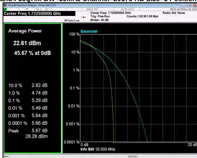
Band4 16QAM BW=10MHz Channel=20350 RB Size=1 Position=#0
