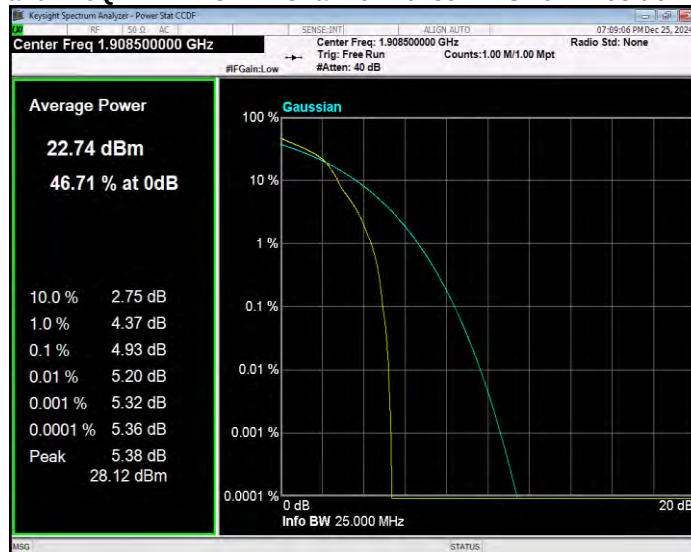
Band2 16QAM BW=5MHz Channel=18625 RB Size=1 Position=#0
