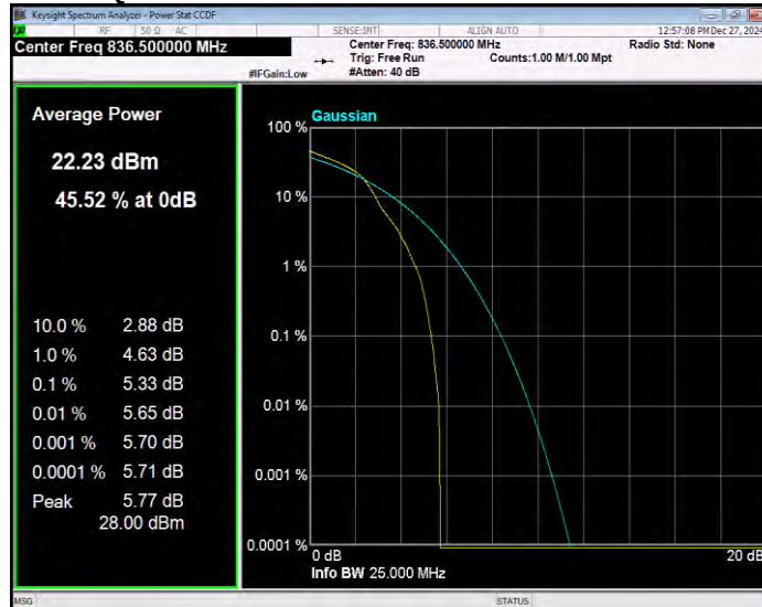
Band5 16QAM BW=3MHz Channel=20635 RB Size=1 Position=#0
