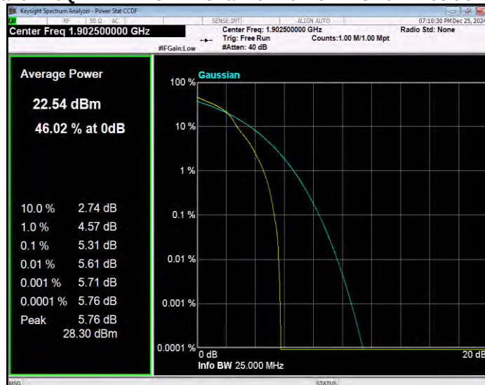
Band2 16QAM BW=20MHz Channel=18700 RB Size=1 Position=#0
