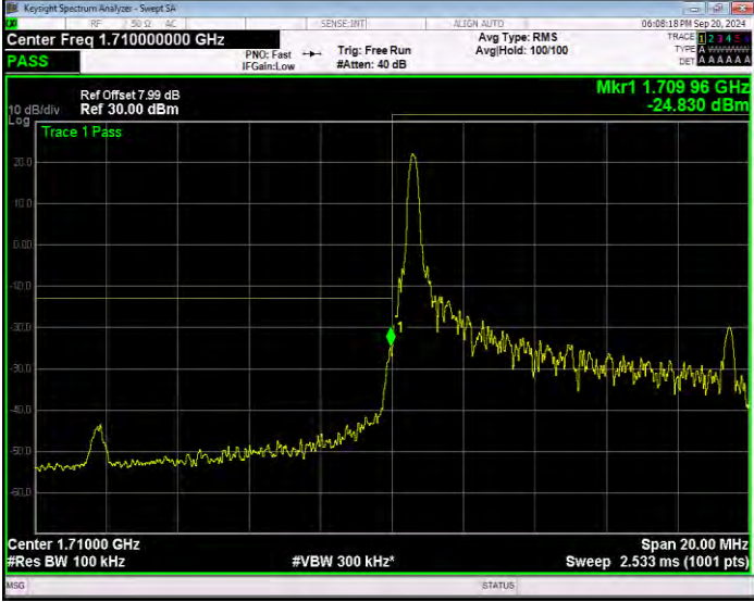
Band66 QPSK BW=10MHz Channel=132022 RB Size=1 Position=#0 Normal
