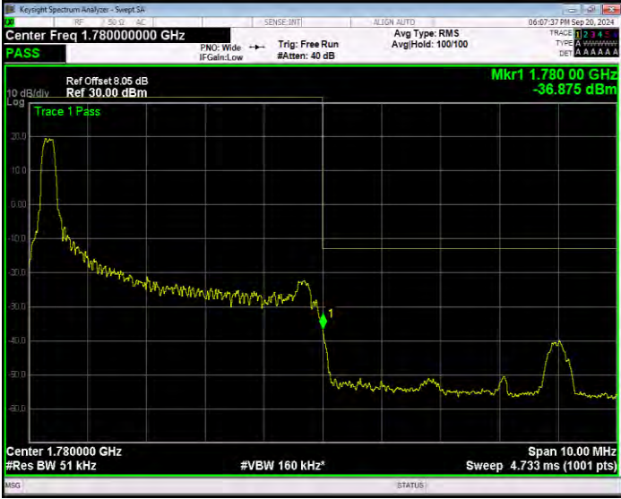
Band66 QPSK BW=5MHz Channel=132647 RB Size=1 Position=#0 Normal
