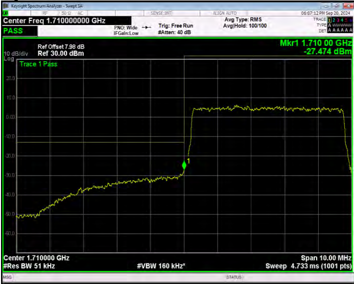
Band66 QPSK BW=5MHz Channel=132647 RB Size=1 Position=#0 Extended
