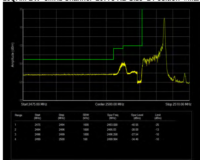
Band7 16QAM BW=5MHz Channel=20775 RB Size=25 Position=#0 Normal
