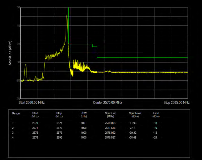
Band7 16QAM BW=5MHz Channel=21425 RB Size=25 Position=#0 Normal
