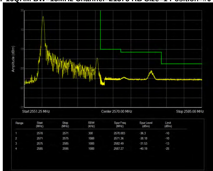
Band7 16QAM BW=15MHz Channel=21375 RB Size=1 Position=#Max Normal
