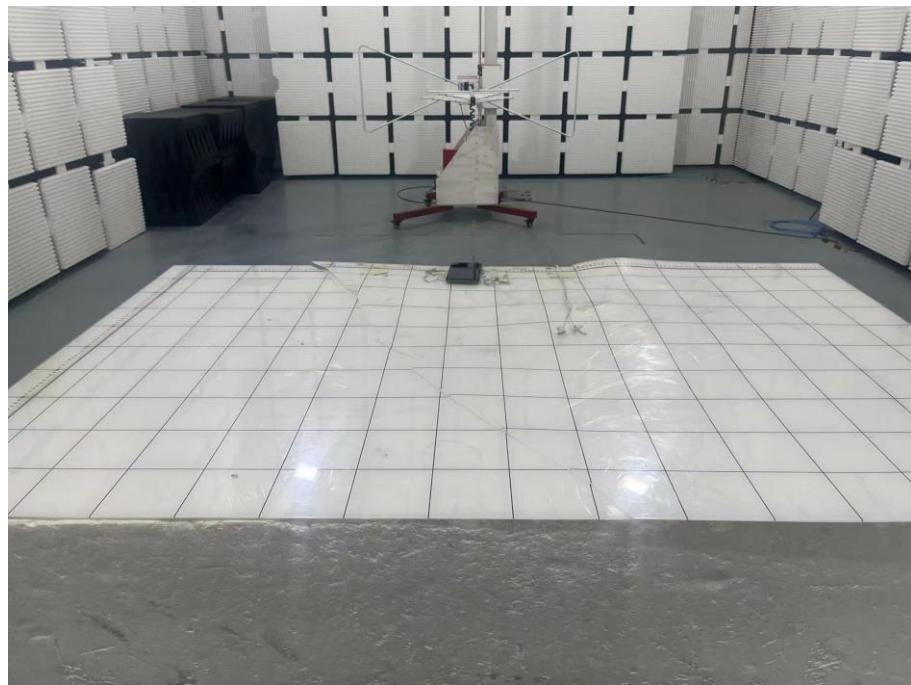
**Set-up for Radiated Emission (RE), Above 1GHz**
