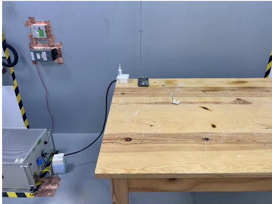
**Set-up for Radiated Emission (RE), Below 1GHz**
