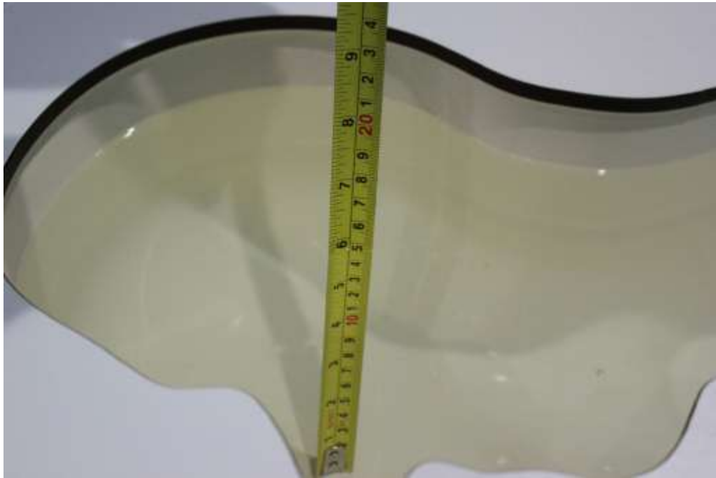
Picture 7-7: Liquid depth in the Head Phantom(5GHz)
