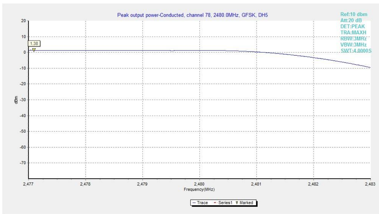
Fig. 3 Maximum Peak Output Power (GFSK, Ch 78)
