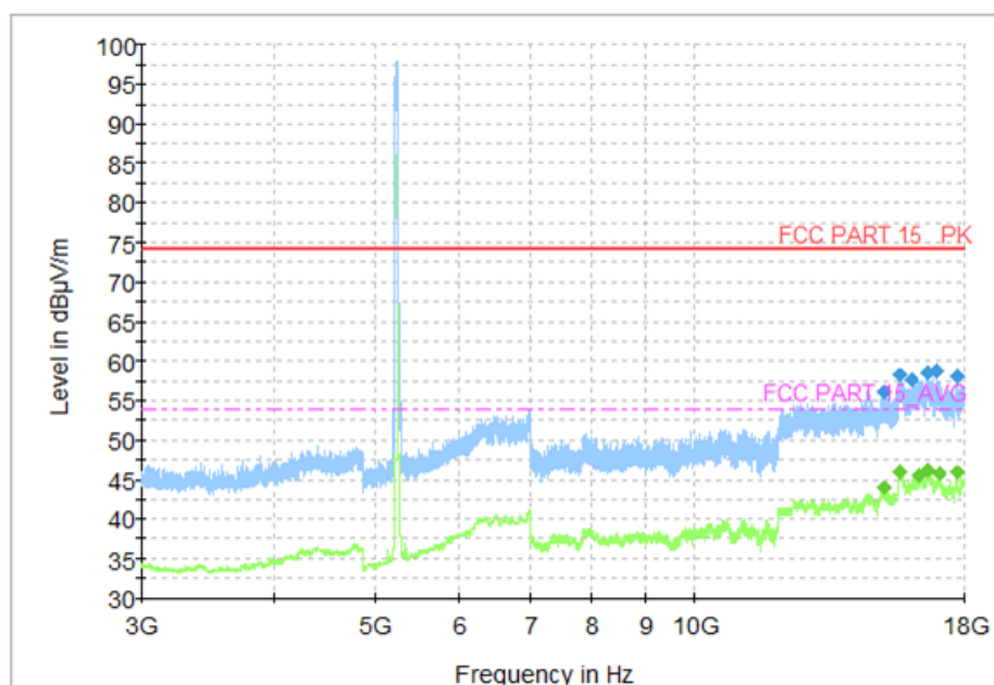
Fig. 90 Transmitter Spurious Emission (802.11n-HT40, CH46 5230MHz, 3 GHz-18 GHz)
