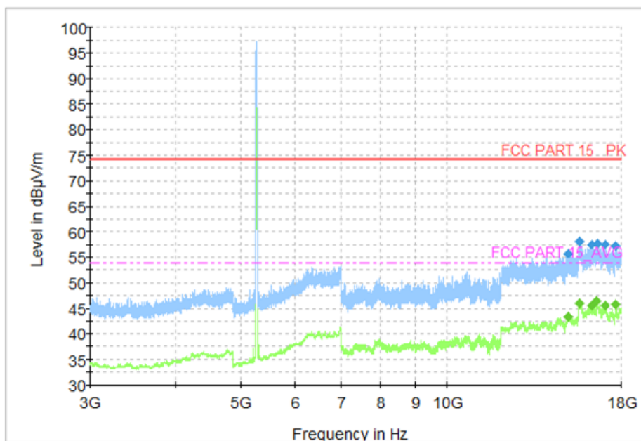
Fig. 70 Transmitter Spurious Emission (802.11a, CH52 5260MHz, 3GHz-18 GHz)
