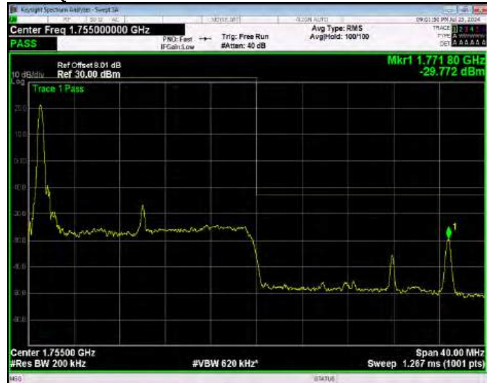
Band4 16QAM BW=20MHz Channel=20300 RB Size=1 Position=#Max Extended
