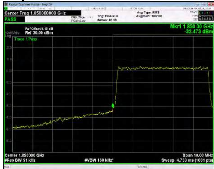
Band2 QPSK BW=5MHz Channel=18625 RB Size=25 Position=#0 Normal
