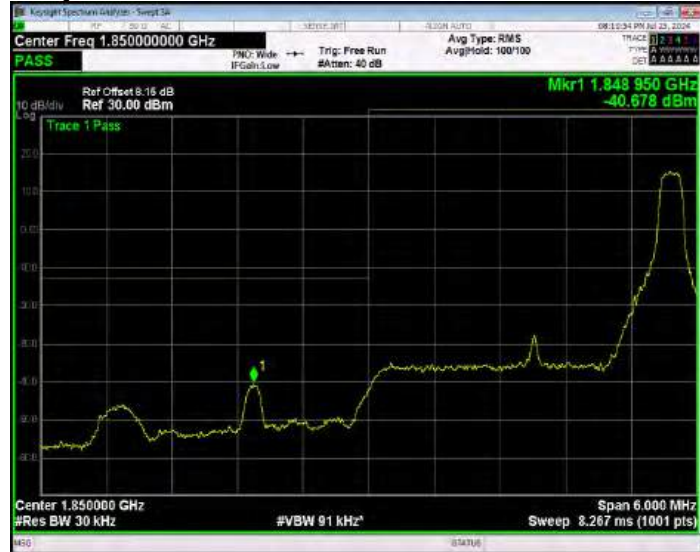
Band2 QPSK BW=3MHz Channel=18615 RB Size=15 Position=#0 Extended
