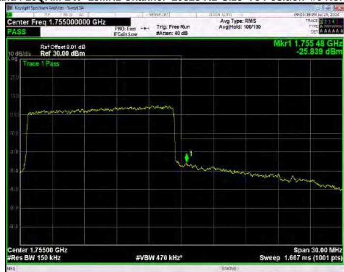
Band4 16QAM BW=15MHz Channel=20325 RB Size=75 Position=#0 Normal
