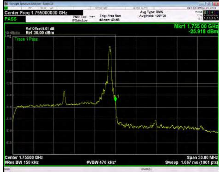
Band4 16QAM BW=15MHz Channel=20325 RB Size=75 Position=#0 Extended
