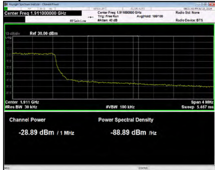
Band2 QPSK BW=3MHz Channel=19185 RB Size=15 Position=#0 Normal
