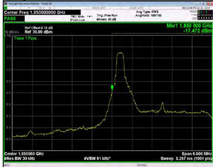
Band2 QPSK BW=3MHz Channel=18615 RB Size=1 Position=#Max Extended
