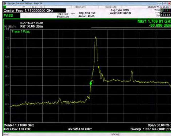
Band4 16QAM BW=15MHz Channel=20025 RB Size=1 Position=#Max Extended
