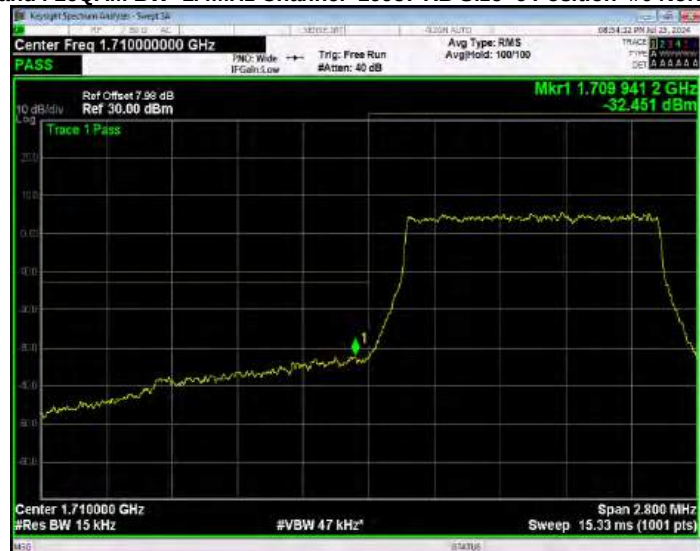
Band4 16QAM BW=1.4MHz Channel=19957 RB Size=6 Position=#0 Normal
