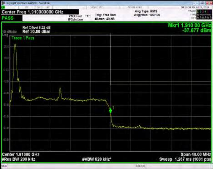
Band2 QPSK BW=20MHz Channel=19100 RB Size=1 Position=#Max Extended
