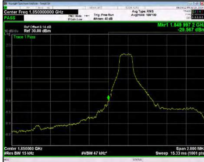
Band2 QPSK BW=1.4MHz Channel=18607 RB Size=1 Position=#Max Extended
