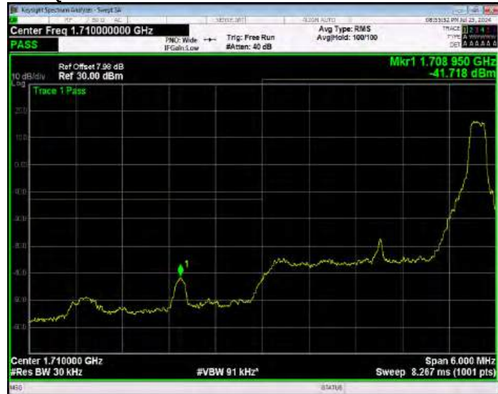
Band4 16QAM BW=3MHz Channel=19965 RB Size=15 Position=#0 Extended
