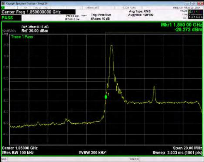
Band2 QPSK BW=10MHz Channel=18650 RB Size=1 Position=#Max Extended
