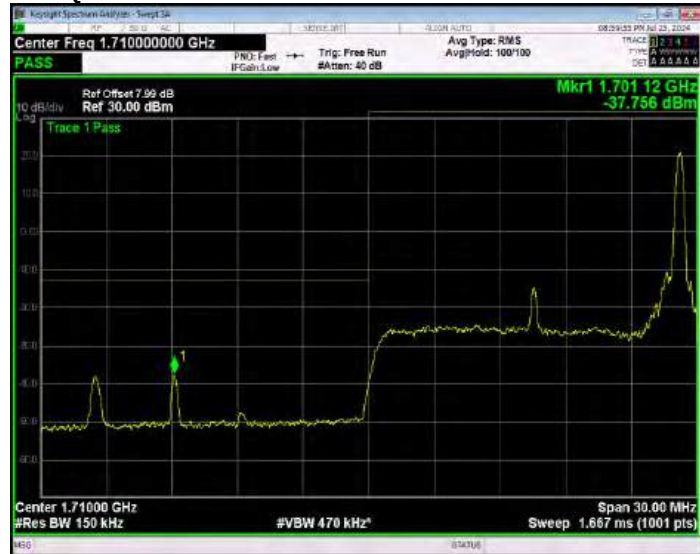
Band4 16QAM BW=15MHz Channel=20025 RB Size=75 Position=#0 Extended
