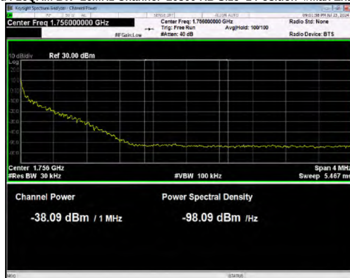
Band4 16QAM BW=20MHz Channel=20300 RB Size=1 Position=#Max Extended
