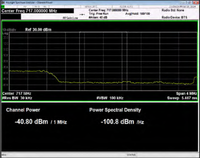
Band17 QPSK BW=5MHz Channel=23825 RB Size=1 Position=#0 Normal
