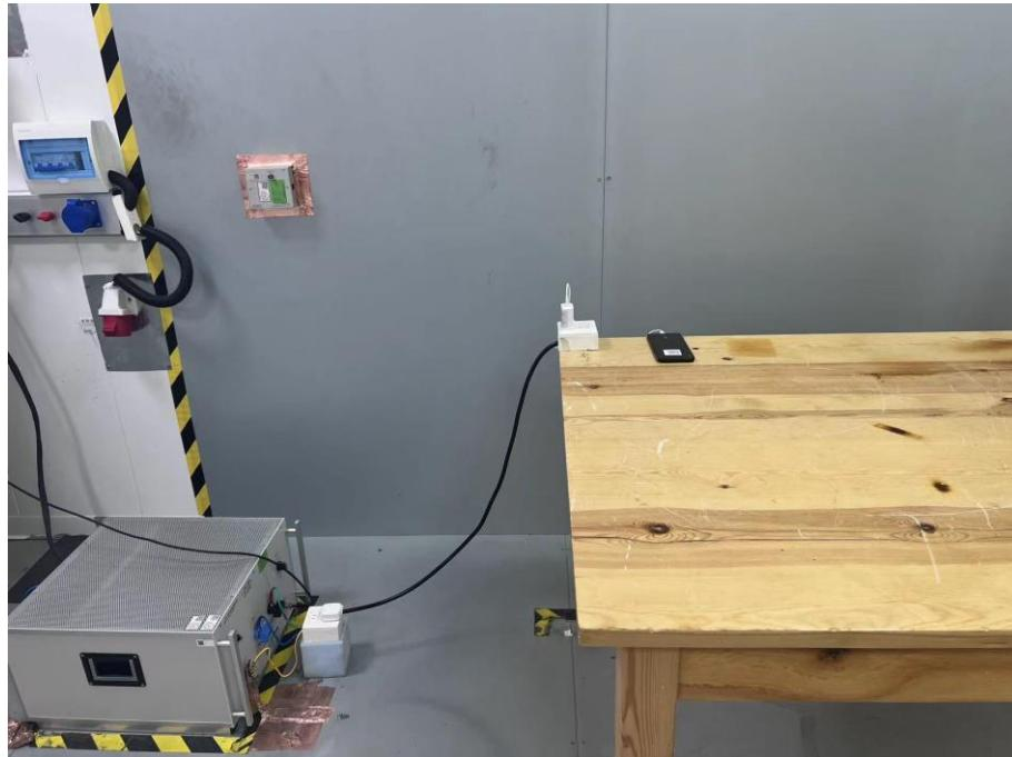
**Set-up for Radiated Emission (RE), Below 1GHz**
