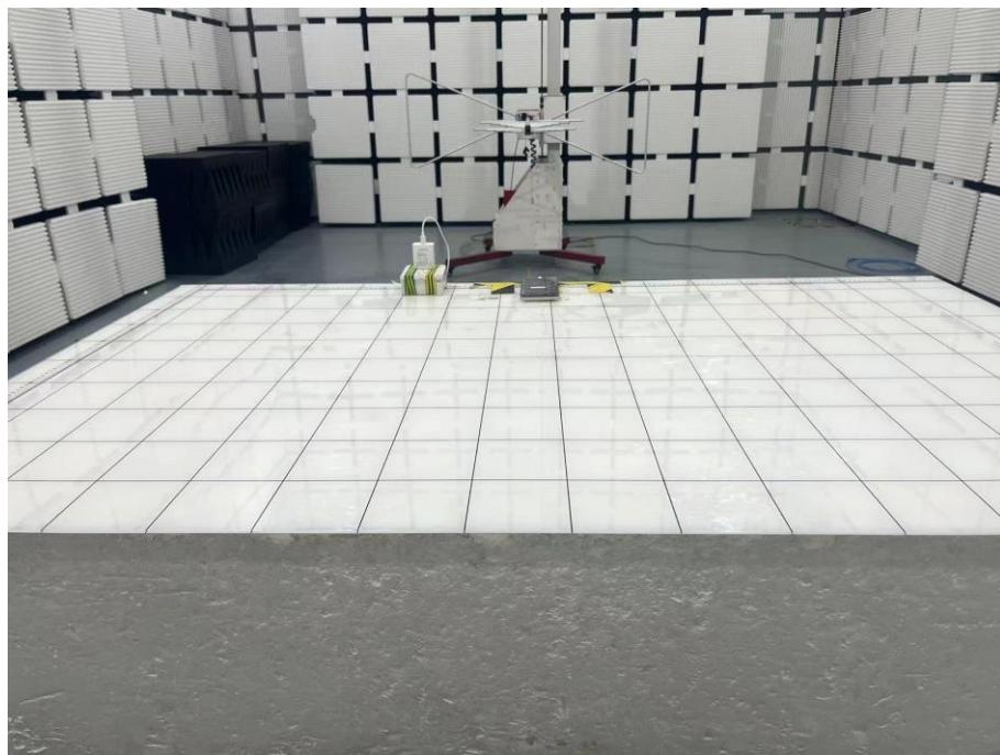
**Set-up for Radiated Emission (RE), Above 1GHz**
