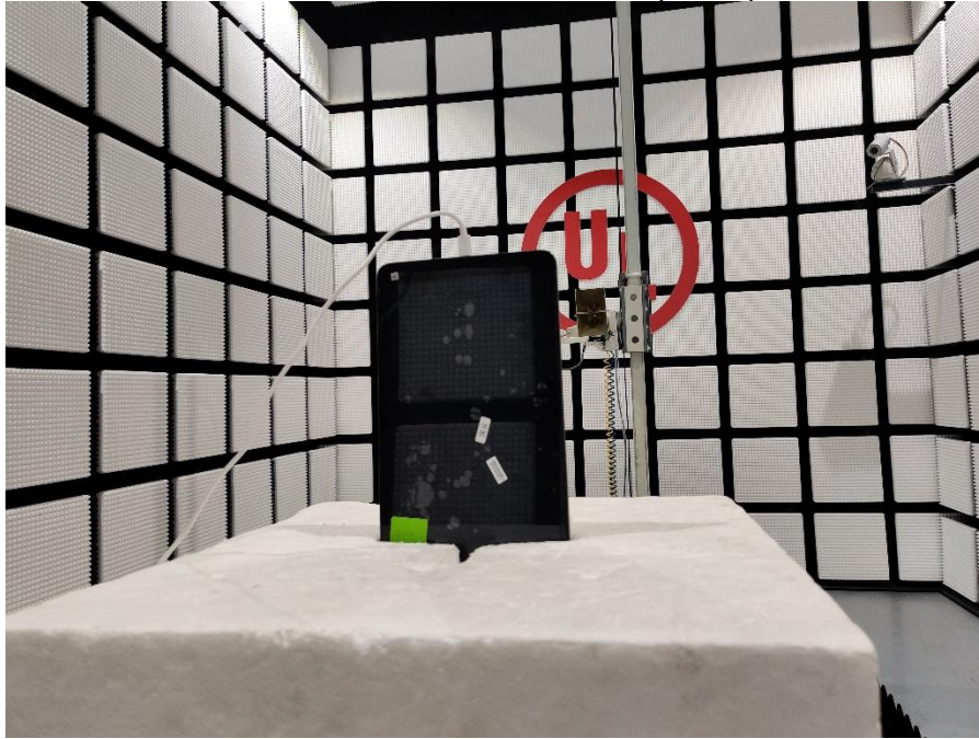
RADIATED RF MEASUREMENT SETUP (30MHz~1GHz)
