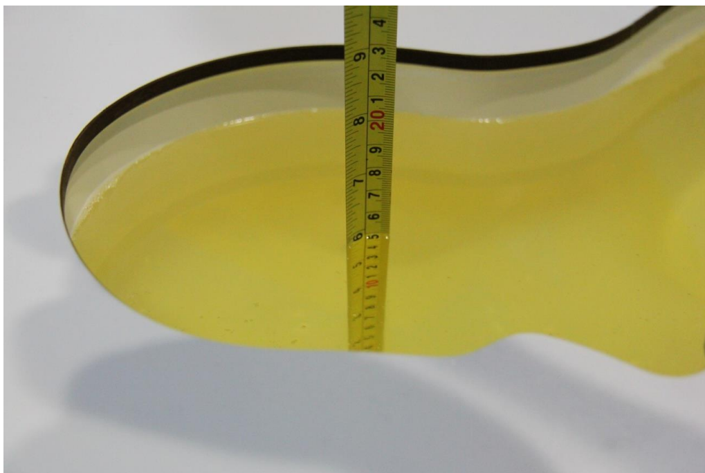
Picture 7-5: Liquid depth in the Head Phantom(2450MHz)
