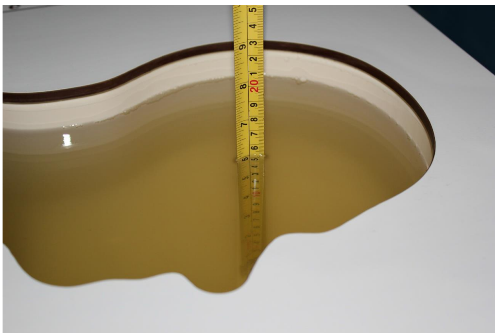
Picture 7-6: Liquid depth in the Head Phantom(2550MHz)
