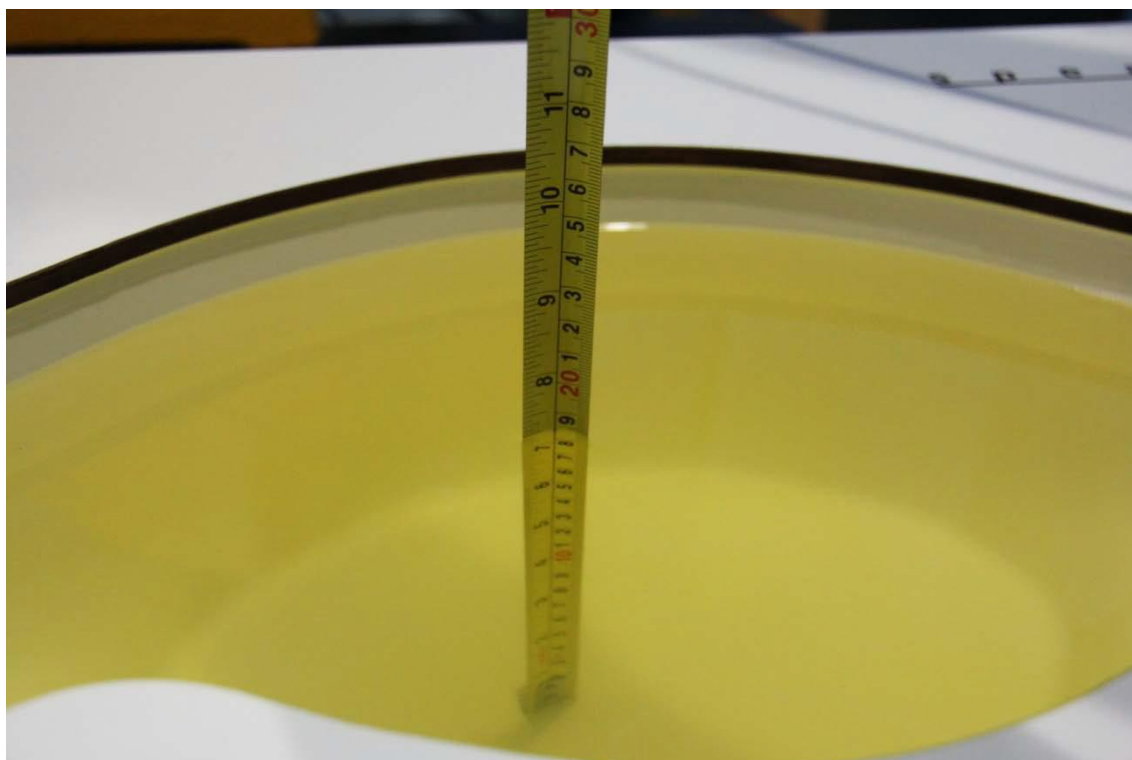
Picture 7-5: Liquid depth in the Flat Phantom(2450MHz)
