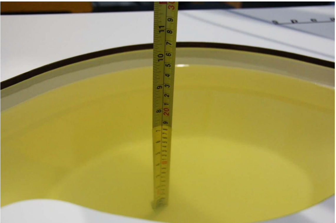
Picture 7-4: Liquid depth in the Flat Phantom(2450MHz)
