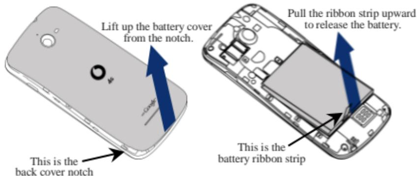
Removing the back cover: **Hold the sides of the phone securely with your left hand; lift up the back cover with your right hand thumbnail, using the notch.**
