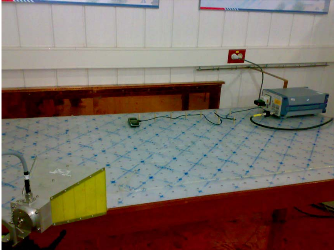
Pic 1 Conducted Emissions Test Setup
