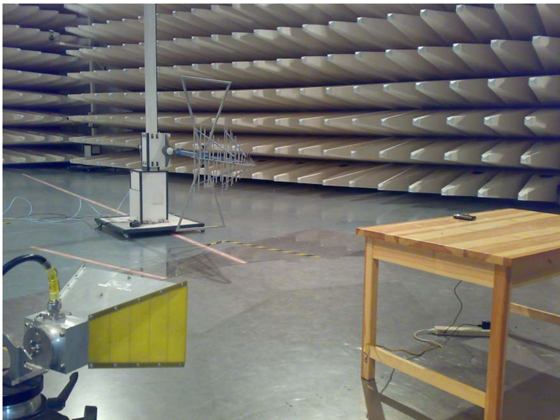
Pic 3 Radiated Emissions Test Setup
