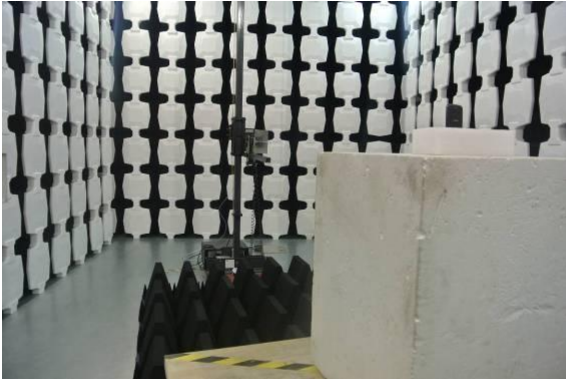
Description: Radiated Spurious Measurement Setup (Above 1GHz)
