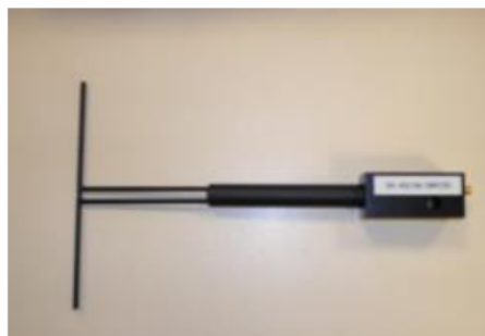
Figure 1 – Satimo COMOSAR Validation Dipole
