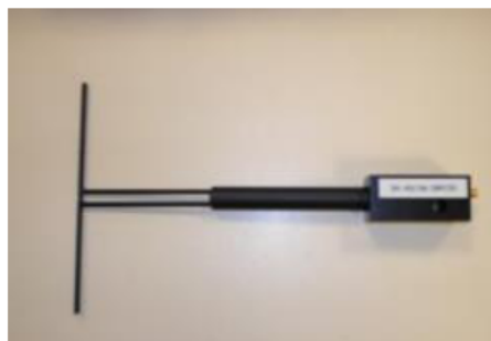
Figure 1 – Satimo COMOSAR Validation Dipole
