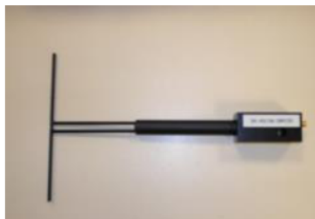
Figure 1 – Satimo COMOSAR Validation Dipole
