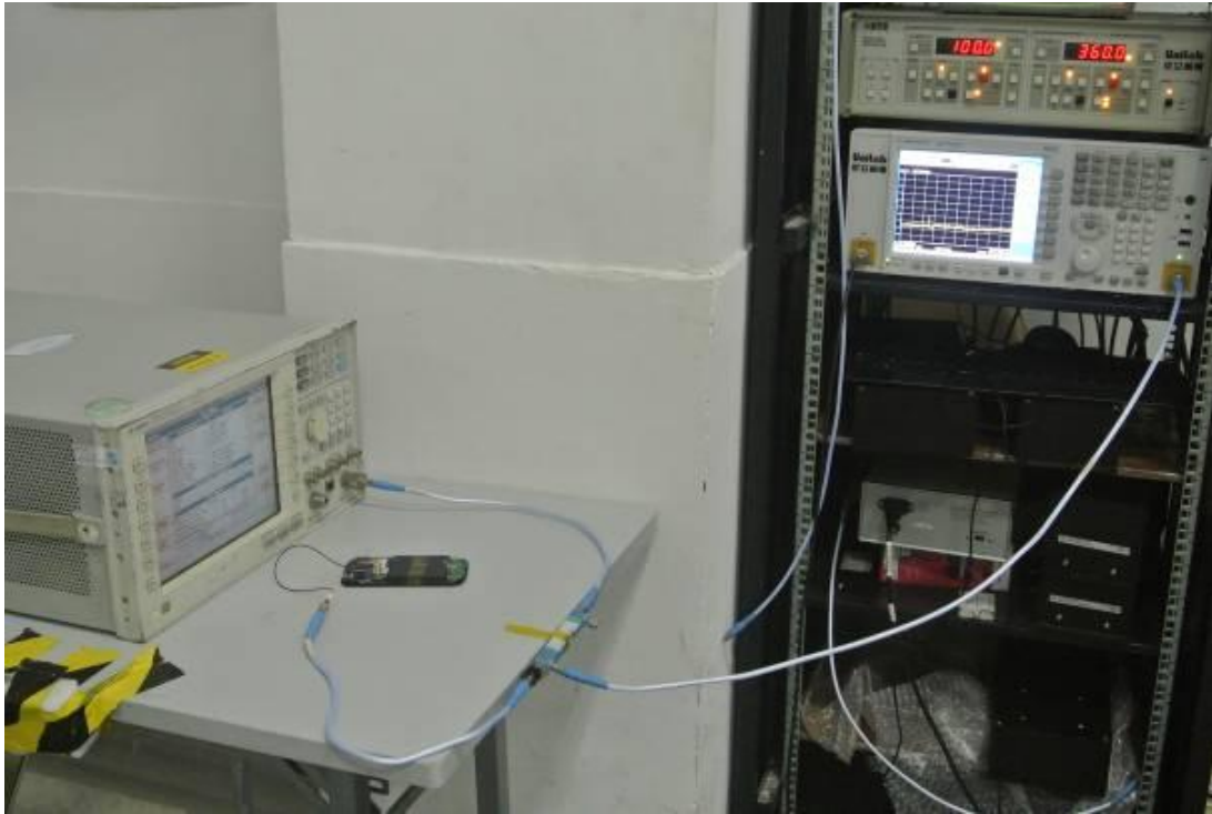
Frequency Stability Under Temperature & Voltage Variations Setup
