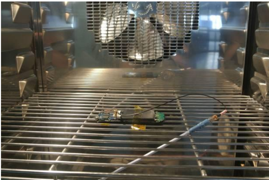
Frequency Stability Under Temperature & Voltage Variations Setup
