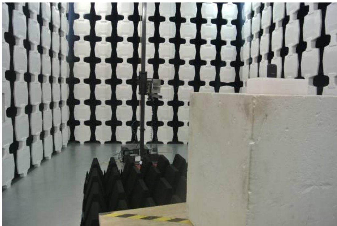
Radiated Spurious Measurement (Above 1GHz), EIRP Test, Receiver Spurious Emission for RSS 132/133/139 Setup
