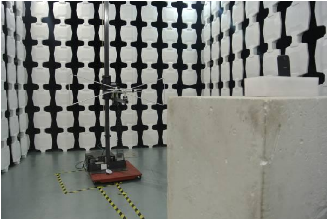
ERP Test, Receiver Spurious Emission for RSS 132/133/139, Radiated Spurious Measurement(Below 1GHz) Setup
