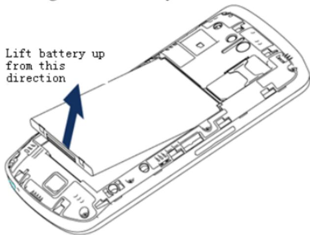
1. With one hand, tightly hold the device face down.
