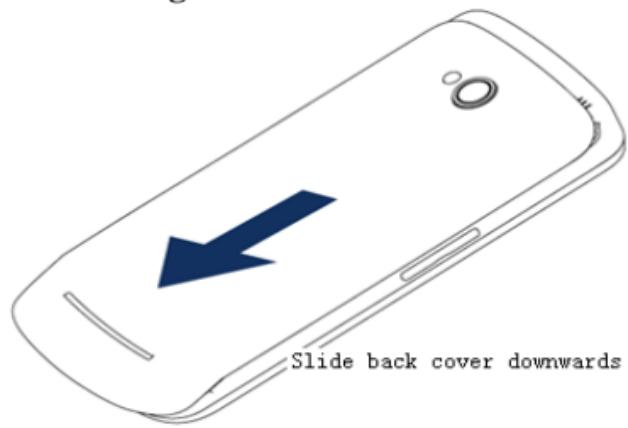
1. With one hand, tightly hold the device face down.
