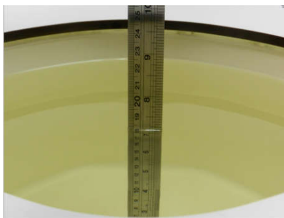
Fig 10.2 Photo of Liquid Height for Body SAR
