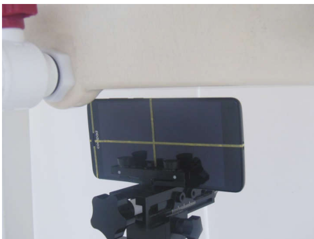
Right Side, Test Separation 10 mm
