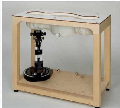
Picture C.8: SAM Twin Phantom
