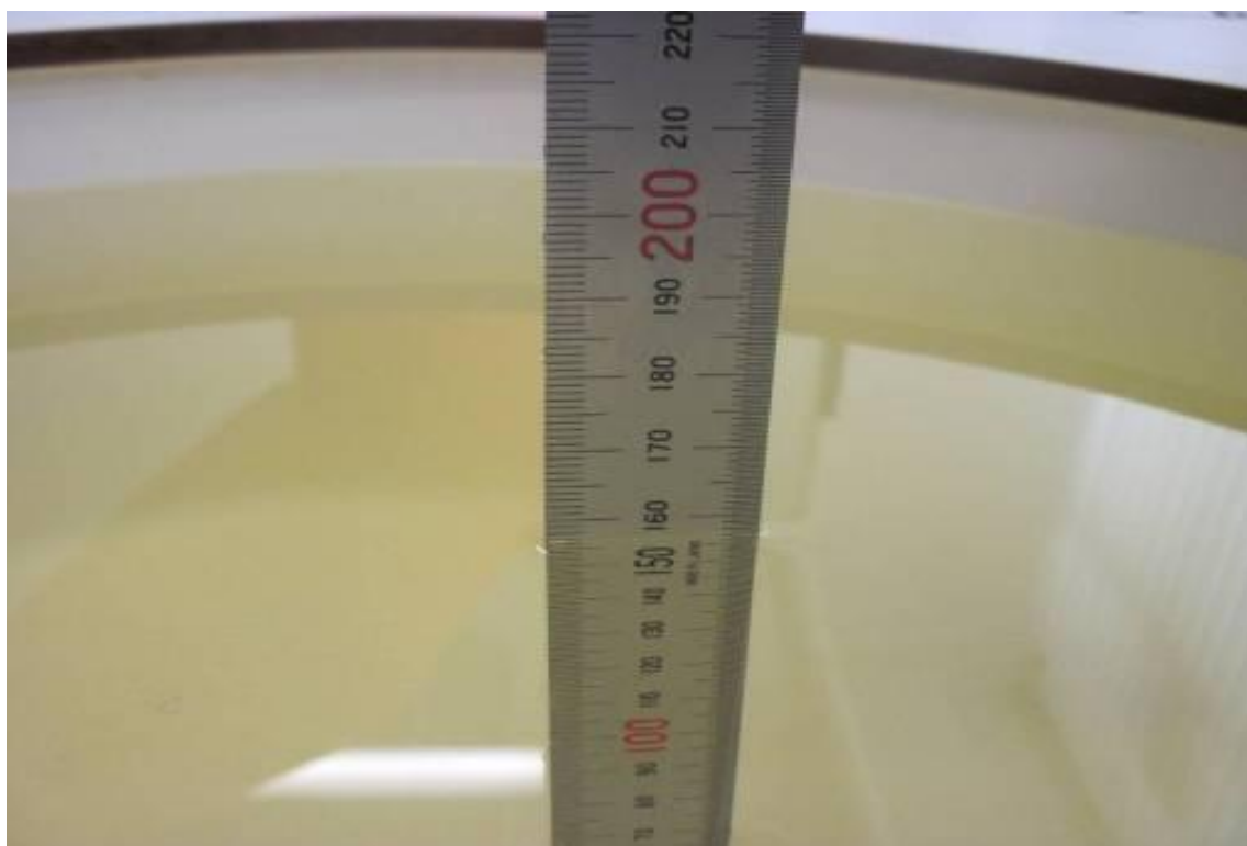
Picture 7-6: Liquid depth in the Flat Phantom (1800MHz)
