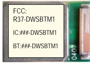
The integrated circuit includes both the RF processor as well as the baseband (BB) processor. All the related Bluetooth protocols that deal with RF modulation, channel hopping sequence and timing, are dealt within the chip. It also has an internal regulator for the core and RF circuitry, and internal VCO and PLL filter.
