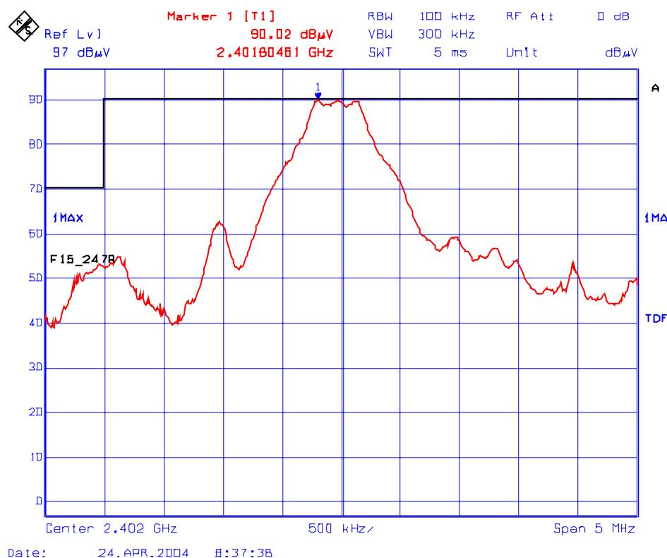
**Plot # 18: Lower Band-Edge Radiated Emissions @ 3 meters, Vertical Polarization**
