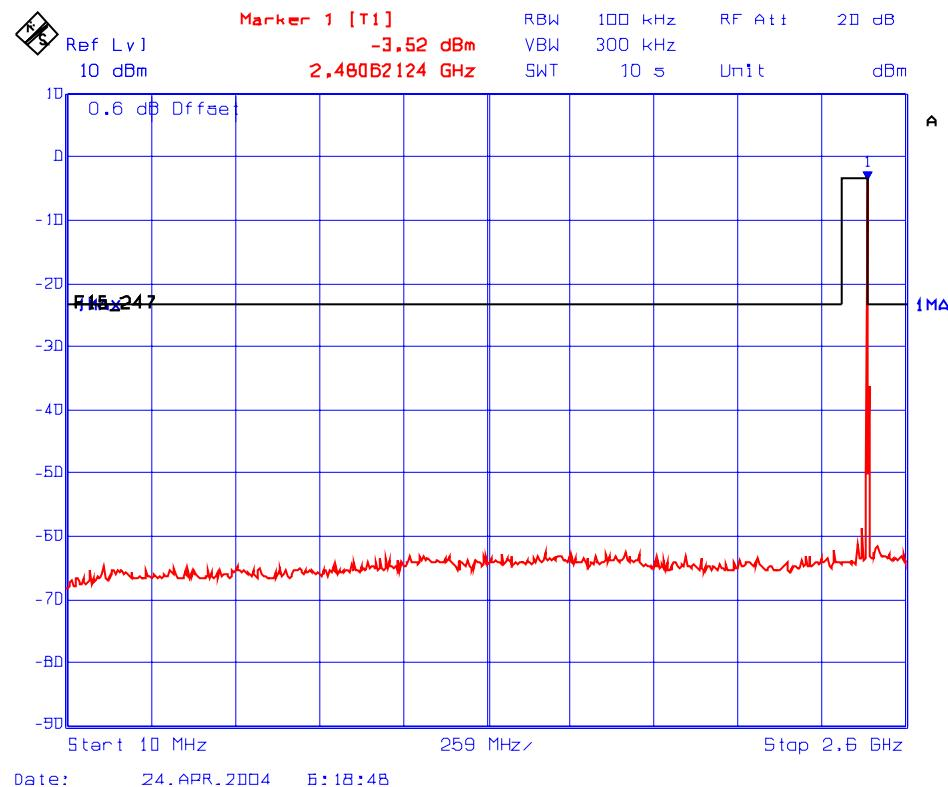
Plot # 13: Spurious RF Conducted Emissions @ Freq. 2480 MHz
