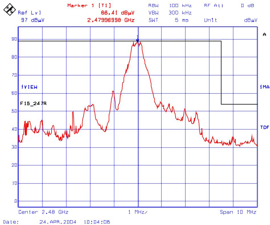
Plot # 20: Upper Band-Edge Radiated Emissions @ 3 meters, Vertical Polarization
