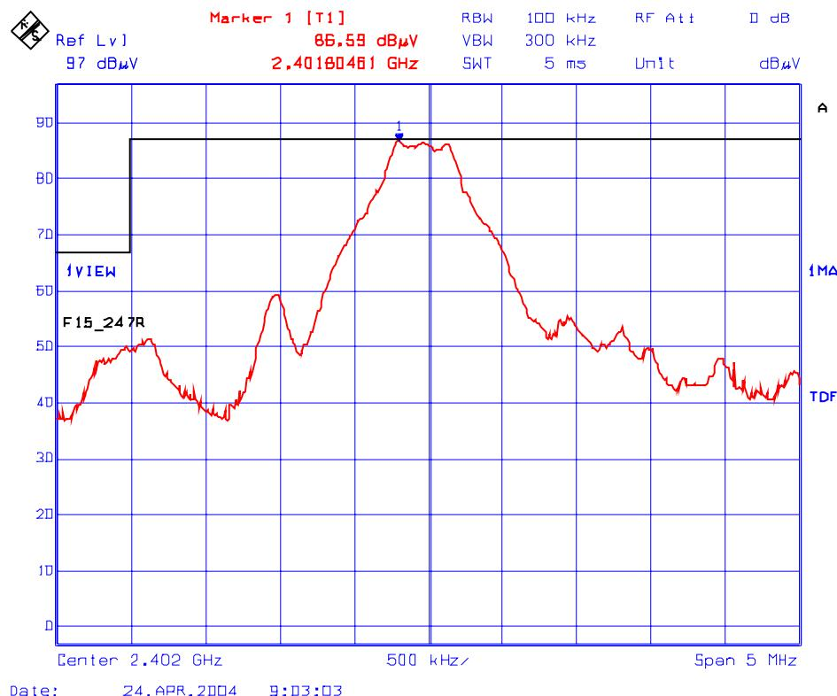
**Plot # 19: Upper Band-Edge Radiated Emissions @ 3 meters, Horizontal Polarization**
