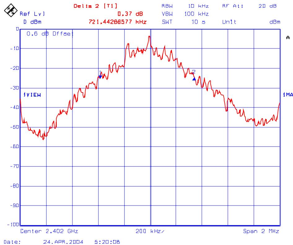
**Plot # 4: 20 dB Bandwidth of 2441 MHz Hopping Channel Frequency**
