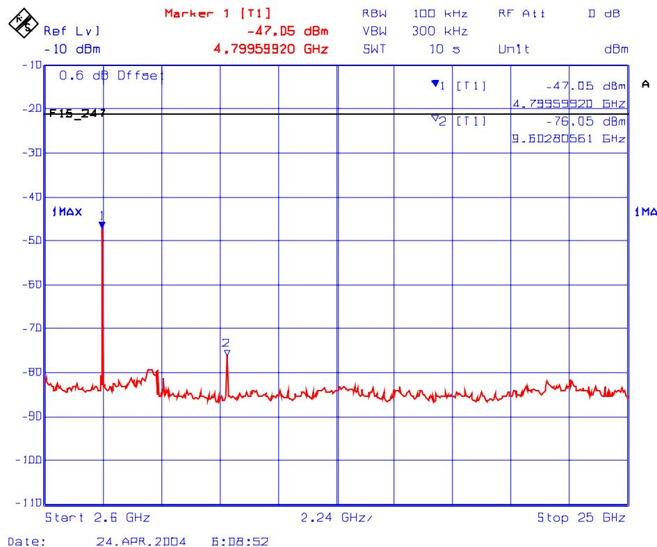
**Plot # 10: Spurious RF Conducted Emissions @ Freq. 2441 MHz**
