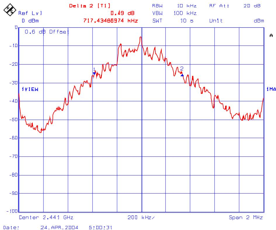
**Plot # 5: 20 dB Bandwidth of 2480 MHz Hopping Channel Frequency**
