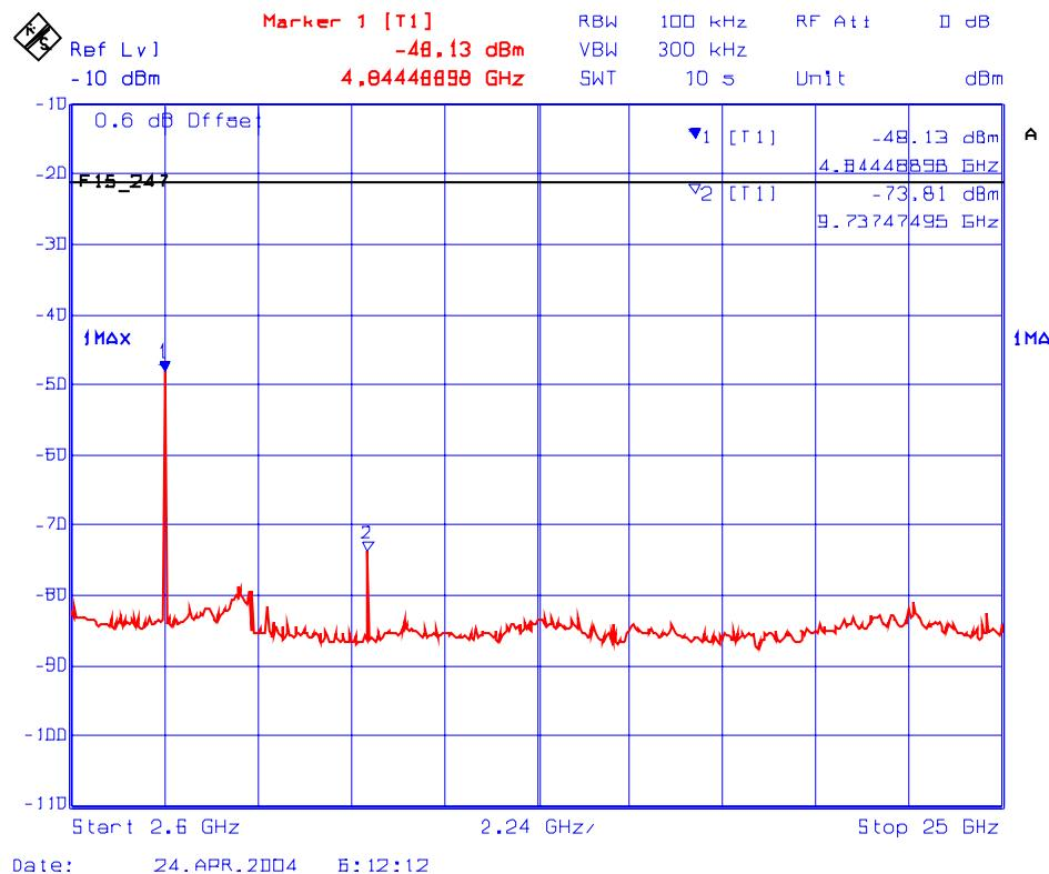
Plot # 12: Spurious RF Conducted Emissions @ Freq. 2480 MHz
