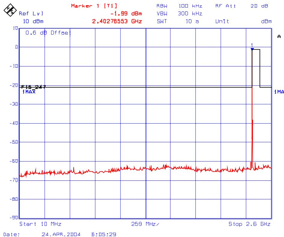
**Plot # 9: Spurious RF Conducted Emissions @ Freq. 2402 MHz**
