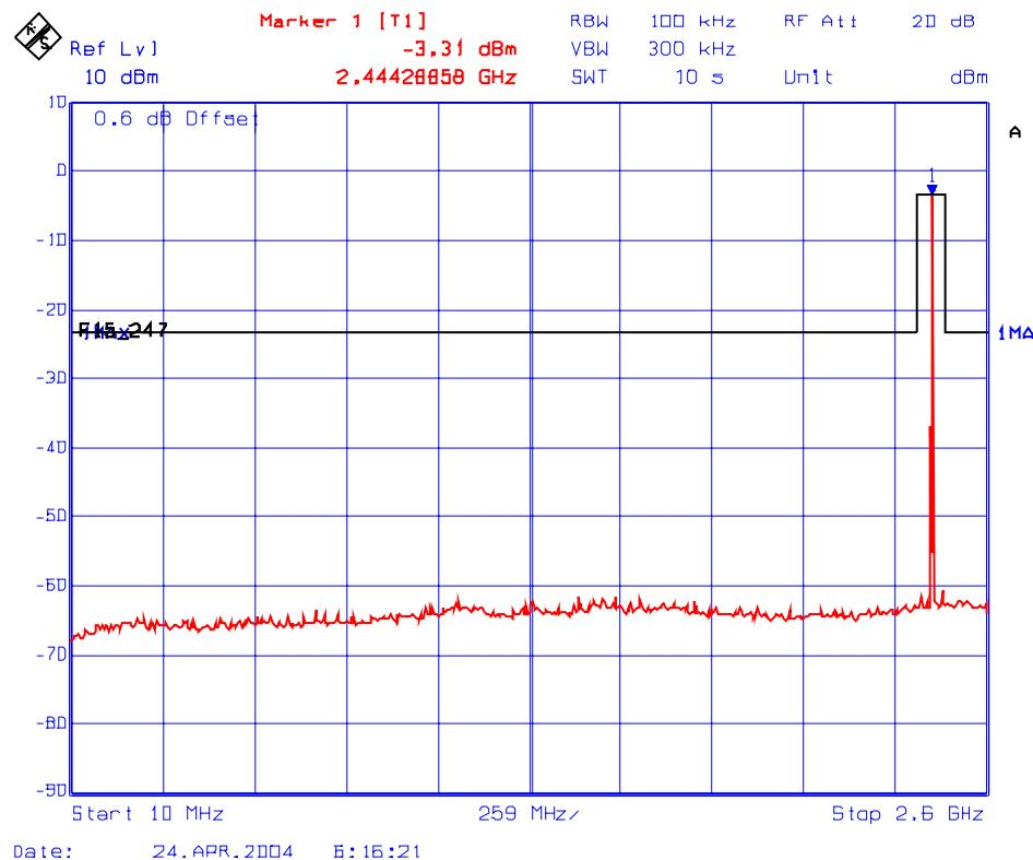
Plot # 11: Spurious RF Conducted Emissions @ Freq. 2441 MHz
