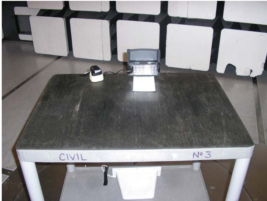
Radiated Emissions Test Setup
