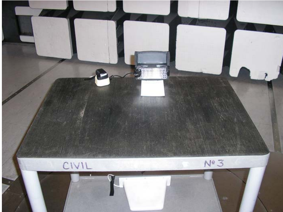
Radiated Emissions Test Setup
