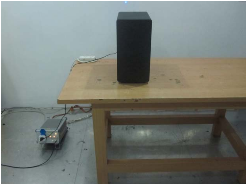
Photo of Setup for Conducted Emission Test
