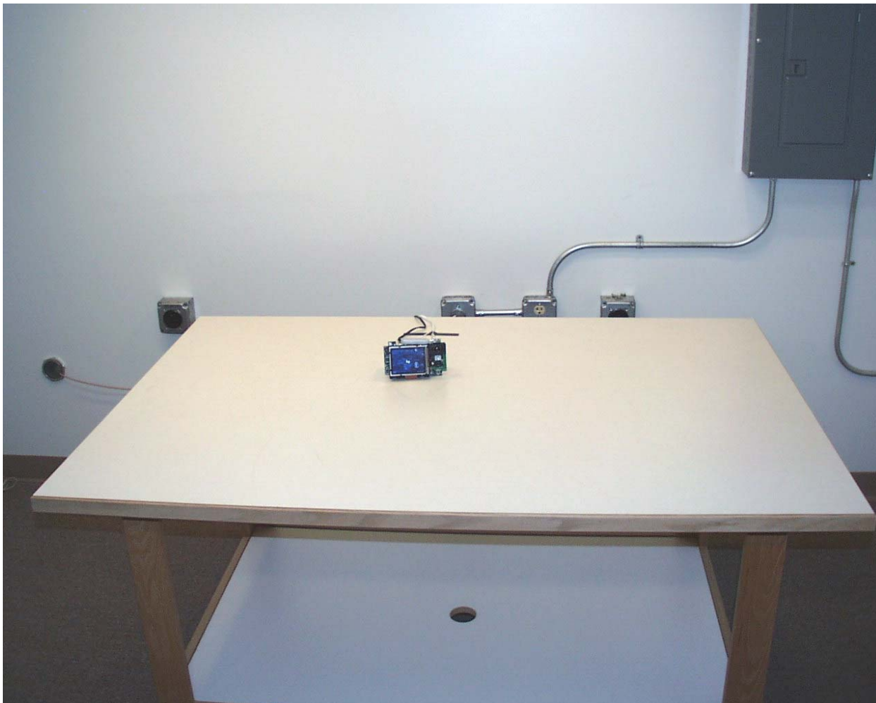
Front View Conducted Disturbance Worst Case Configuration
