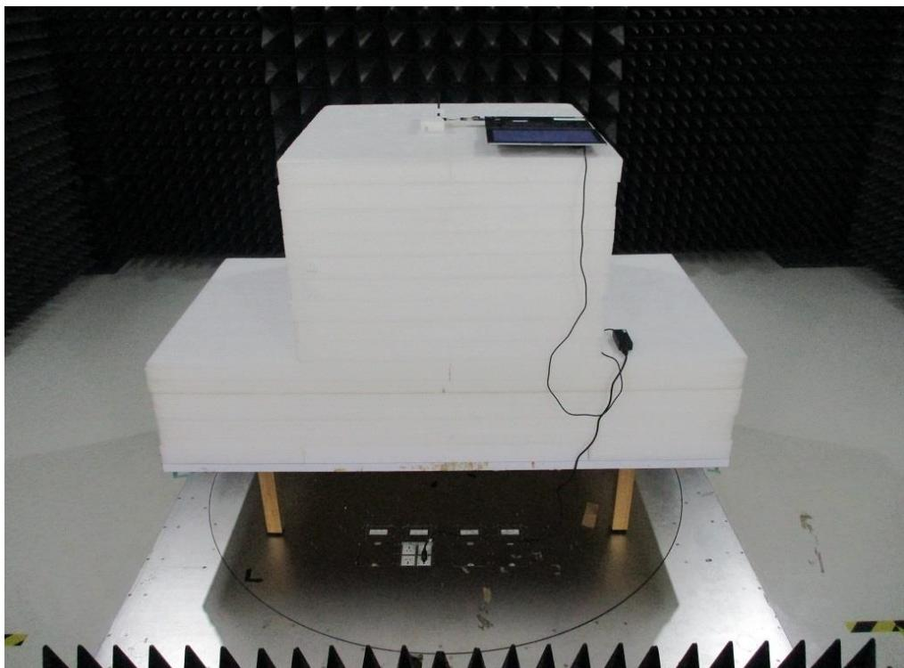
**Radiated Emission Above 1GHz Test**
