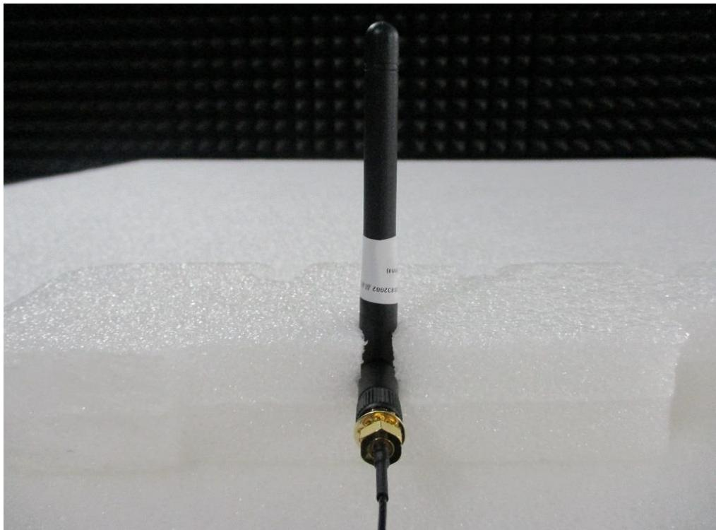
**Radiated Emission Above 1GHz Test**
