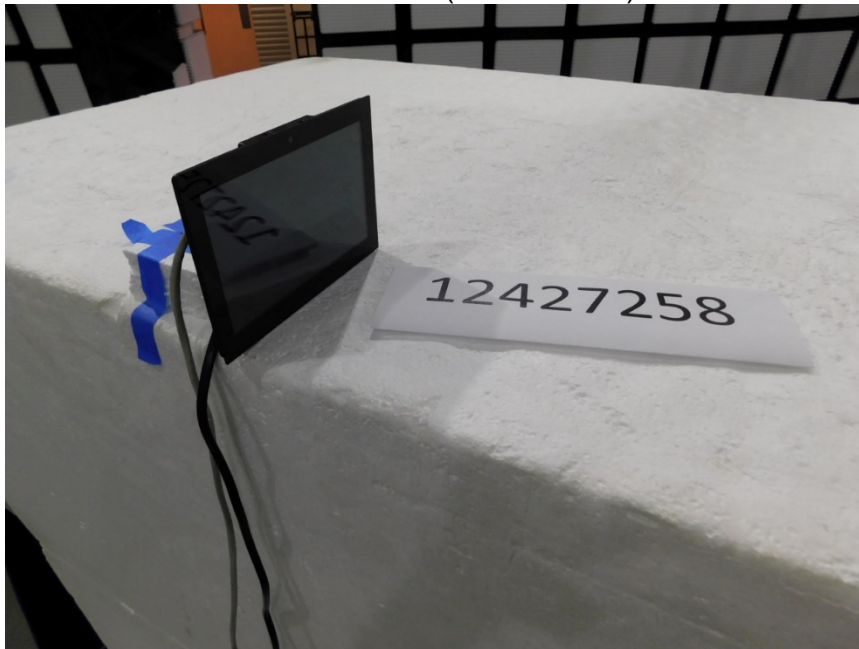
RADIATED SPURIOUS PHOTO (Y Orientation)
