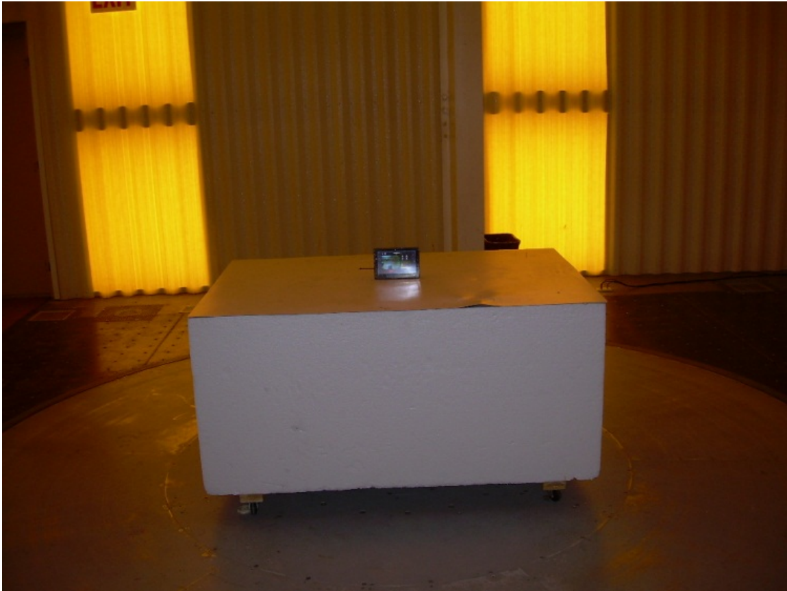
Photograph 1 – Front View Radiated Spurious Emissions – POE Configuration
