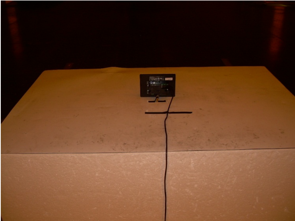
Photograph 2 – Back View Radiated Spurious Emissions – POE Configuration
