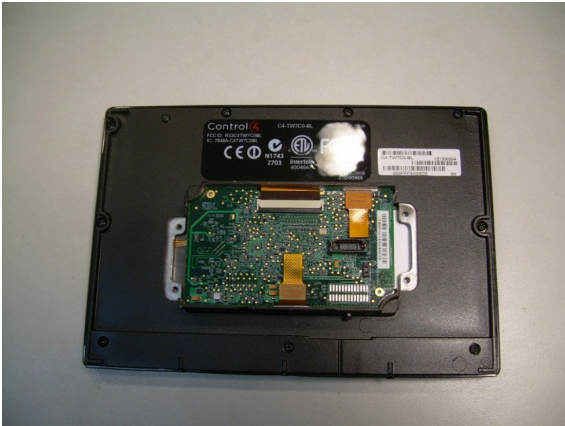
Photograph 17 – Back View of Display Unit with Cover Removed
