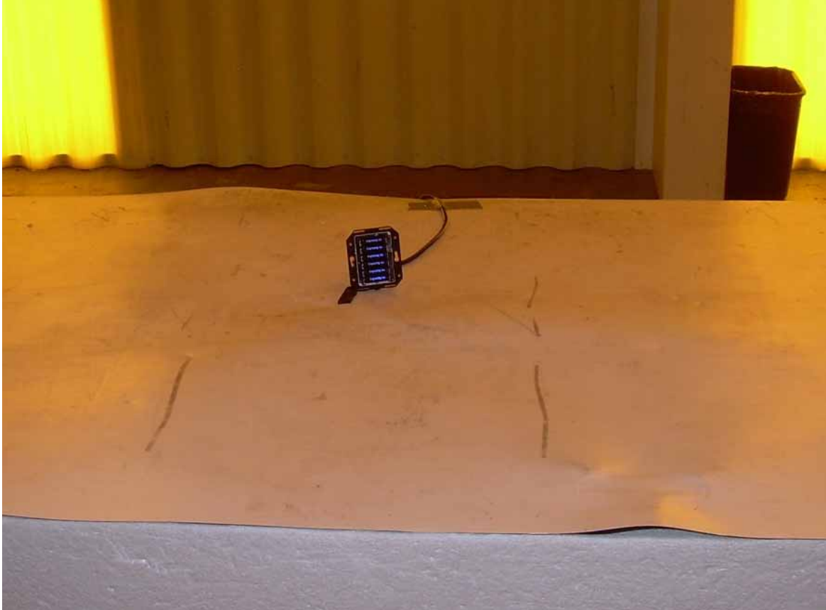
Photograph 1 – Front View Radiated Disturbance Worst Case Configuration
