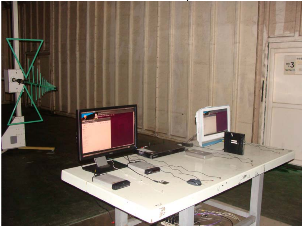
Front View of Radiated Test – Dipole antenna
