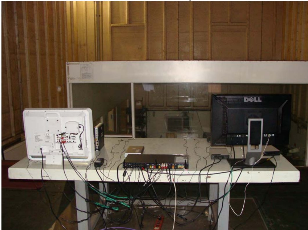
Back View of Radiated Test - Dipole antenna
