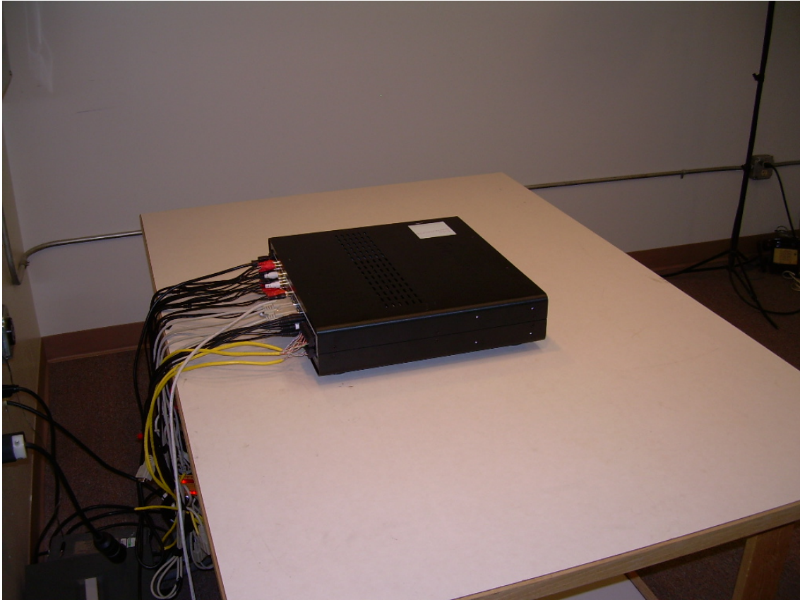
Back View Conducted Disturbance Worst Case Configuration
