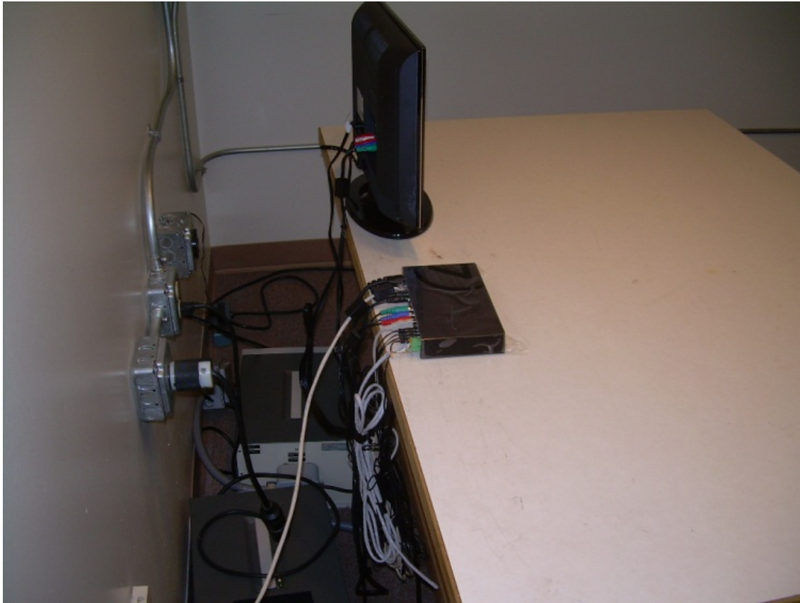
Back View Conducted Disturbance Worst Case Configuration
