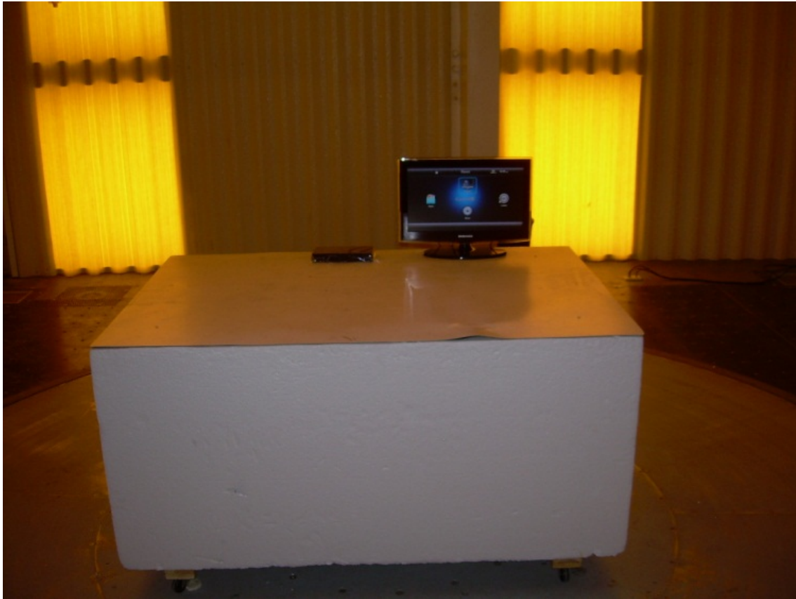
Front View Radiated Disturbance Worst Case Configuration
