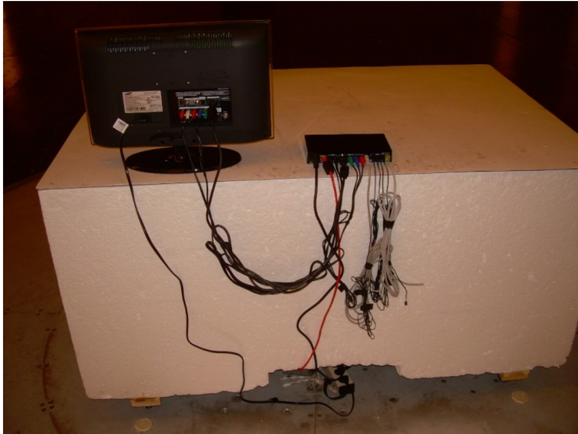
Back View Radiated Disturbance Worst Case Configuration
