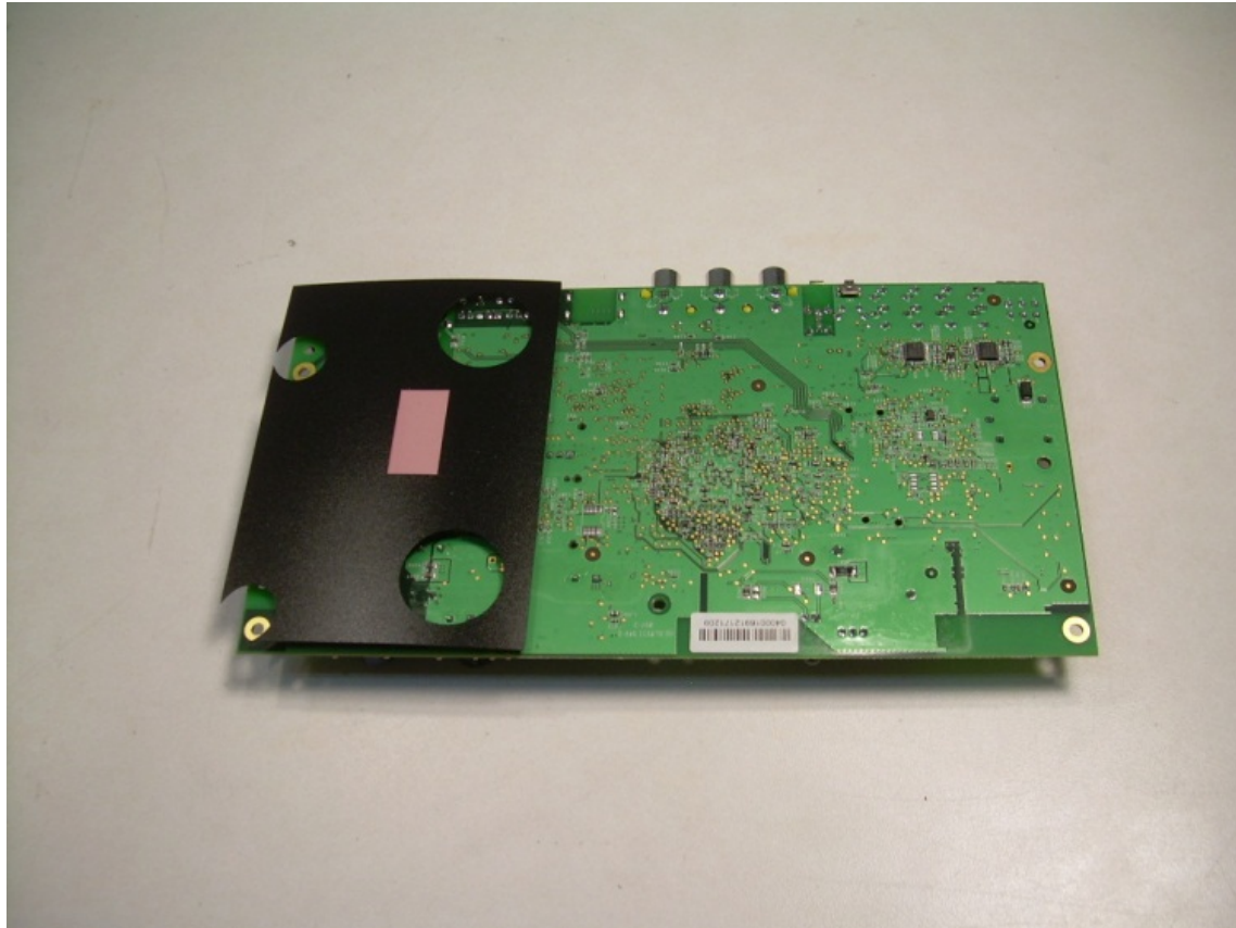
View of the Bottom Side of the PCB – Insulator in Place
