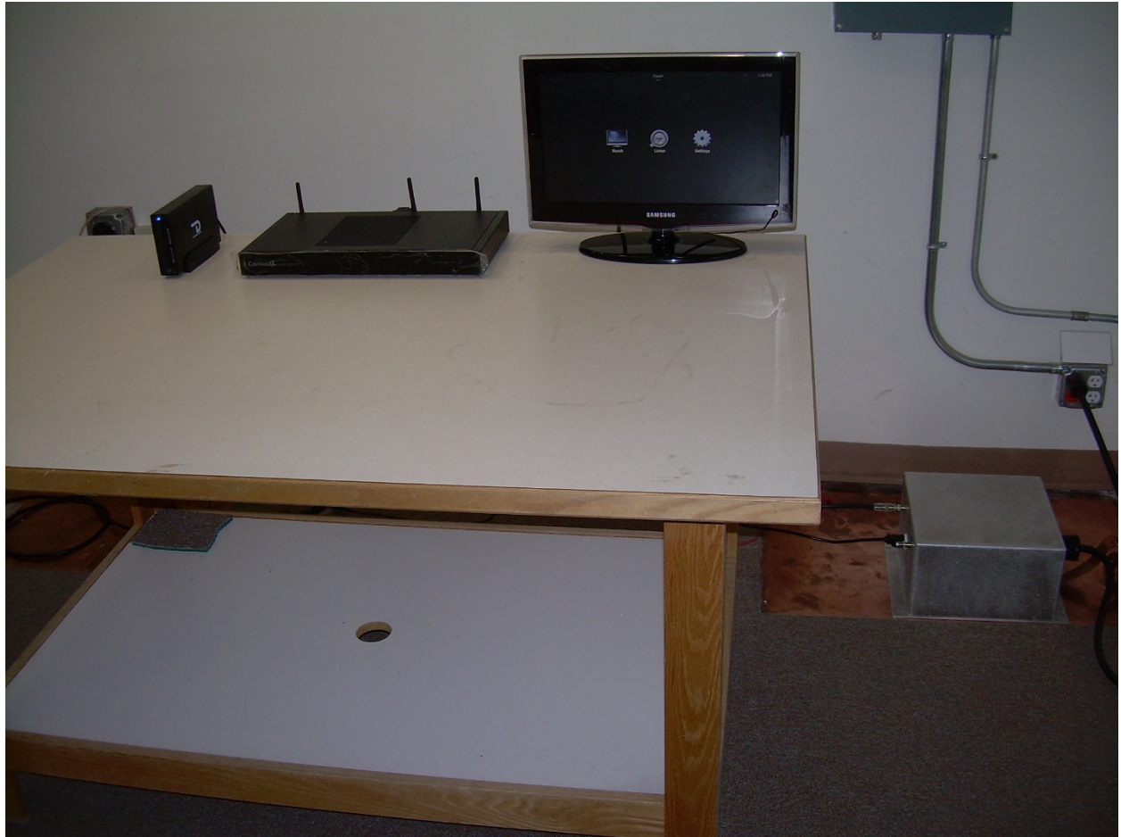
Front View of the Conducted Emission Setup
