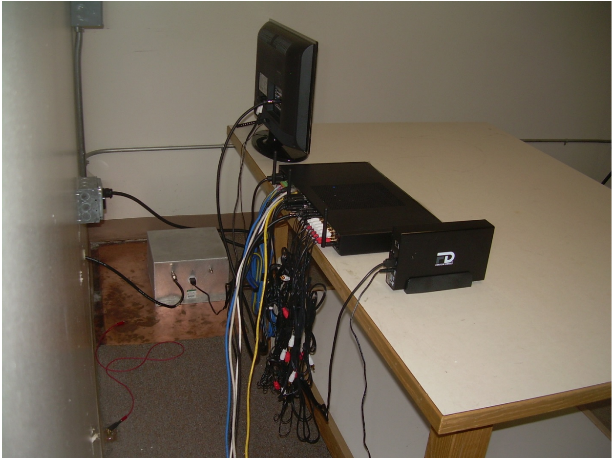
Back View of the Conducted Emission Setup
